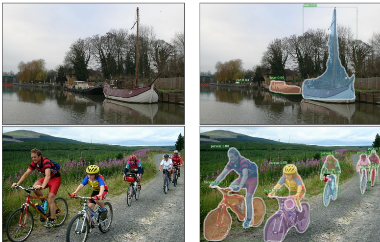
Figure 3.4: Instance-aware semantic segmentation examples with images of the Pascal VOC dataset (Everingham et al., 2010) using Mask-RCNN He et al. (2017). Note that different instances of the same category, e.g., car and person, show individual colors indicating different object identifiers.
