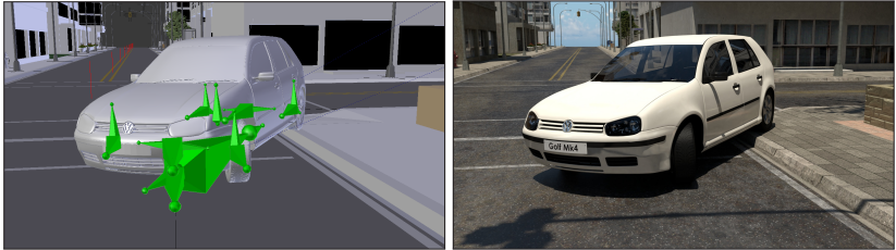
(b) Vehicle rig adjusted to the motion trajectory. The rig controls the correct placement (rear left wheel) and the correct steering (front left wheel).
