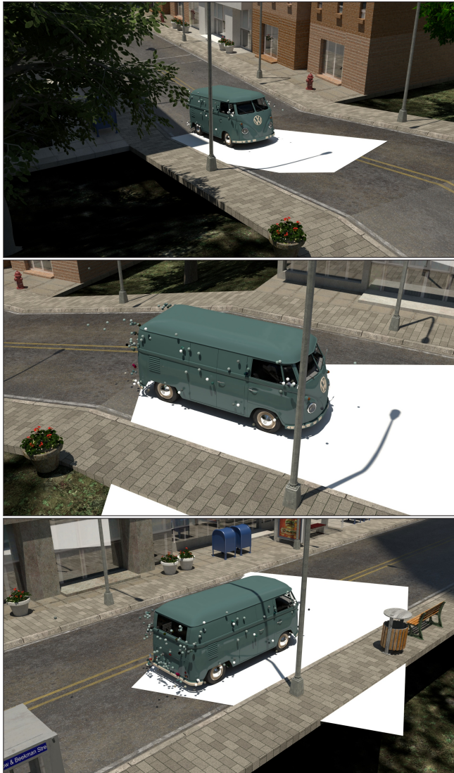
Figure A.4: Reconstruction results using the trajectory estimation method described in section 6.4.2. The small spheres represent triangulated object points and the white planes the local ground approximations.
