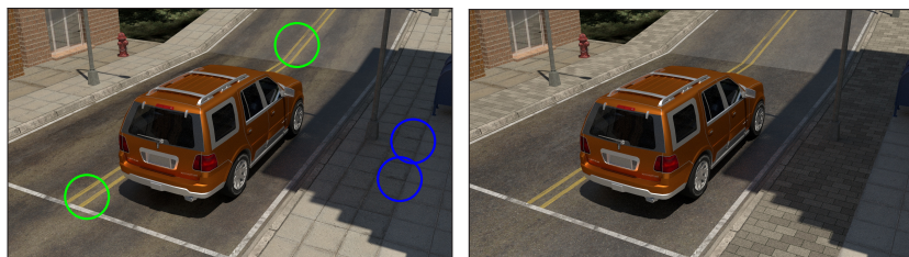
(a) Environment model with repetitive textures. A few examples are emphasized with green and blue. (b) Environment model with procedurally generated textures.
