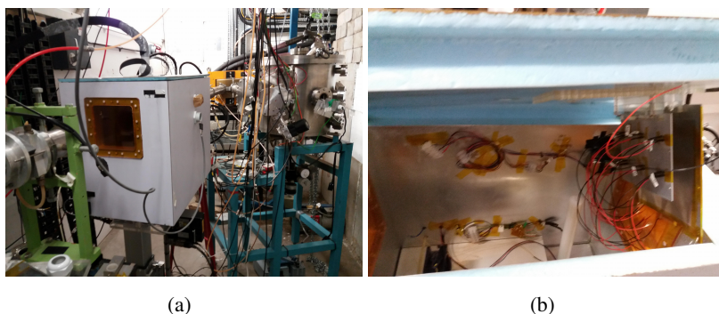
Figure 1. (a) The high intensity area of the MC40 cyclotron with the temperature controlled chamber. (b) The interior of the temperature controlled chamber, viewed from the side. The aluminium plate used to mount the diodes is visible on the right.
