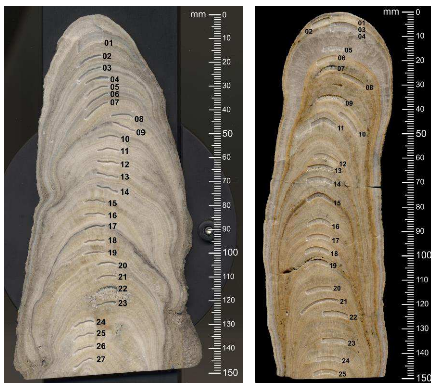
Figure 4.6: Locations of the samples extracted from stalagmite VML22 (left) and VSMS2 (right) for XRD analysis, numbered in black.
