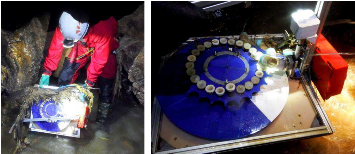
Figure 2.11: Prototype 1.0 installed in Sang Ma Sao cave destroyed by the cave river during an exceptionally high flow event after a couple of days of strong rain (photo: Prof. Dr. Thomas Neumann; 6 th of October, 2015).
