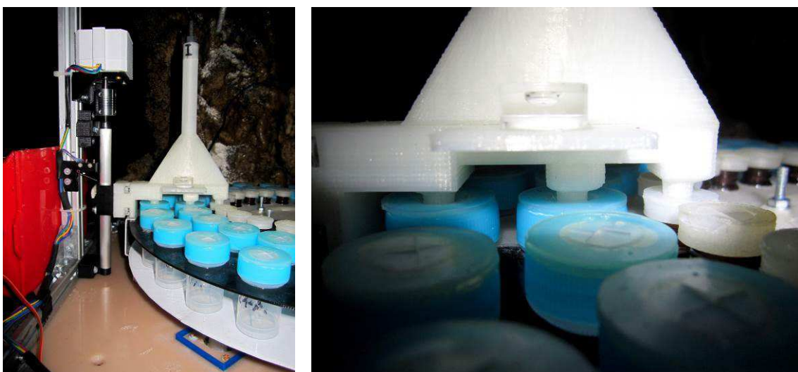
Figure 2.9: Initial setup of Prototype 1.0 installed in Ma Le 2 cave right after the start of the first sampling cycle (left) showing no signs of errors and close-up of the “drip divider” with its nozzles successfully piercing the septa of the sample flasks. (Photo: A. Hartmann; 22 nd of July, 2015).
