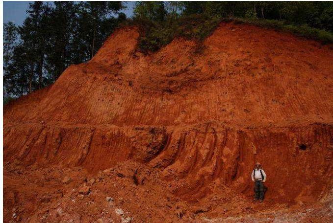
Figure 3.10: Picture illustrating the great depth to which the soils in the study area are developed and their intense red-brown colour. Picture taken at the southwest end of Dong Van City (April 4 th , 2016).
