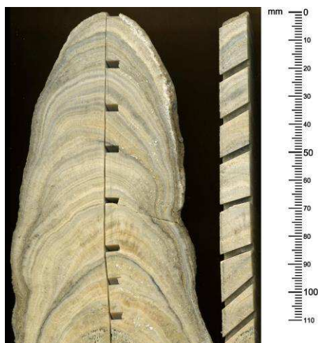
Figure 4.1: Slab of stalagmite VML22 after extraction of samples for U/Th dating using a band-saw. To minimize the error due to subsample mixing the cuts follow the inclination of the growth laminae (left: top view; right: perpendicular view on the cutting edge).
