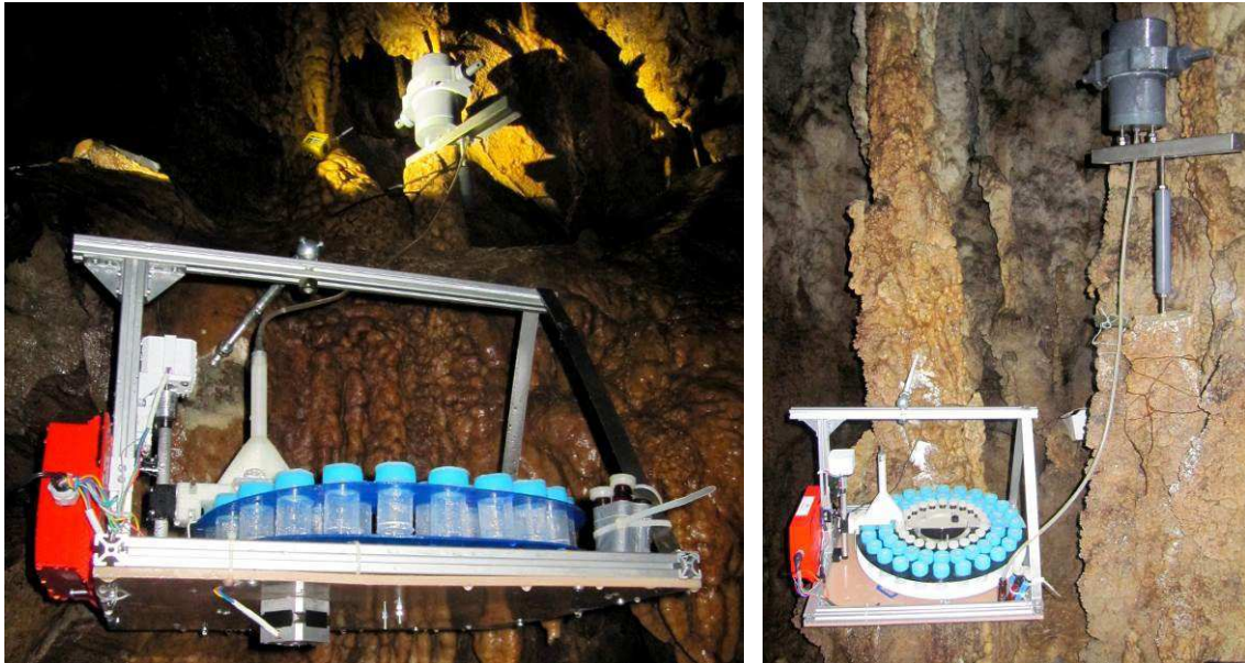
Figure 2.8: Dripwater collection system consisting of the Prototype 1.0 dripwater autosampler and the dripwater container including the Stalagmate drip rate logger, installed inside Sang Ma Sao cave (left) and Ma Le 2 cave (right). In the left picture, the yellow box on the left-hand side of the dripwater collector is the Tinytag TGP-4500 T/RH logger. (Photos: A. Hartmann; 22 nd and 29 th of July, 2015, respectively).
