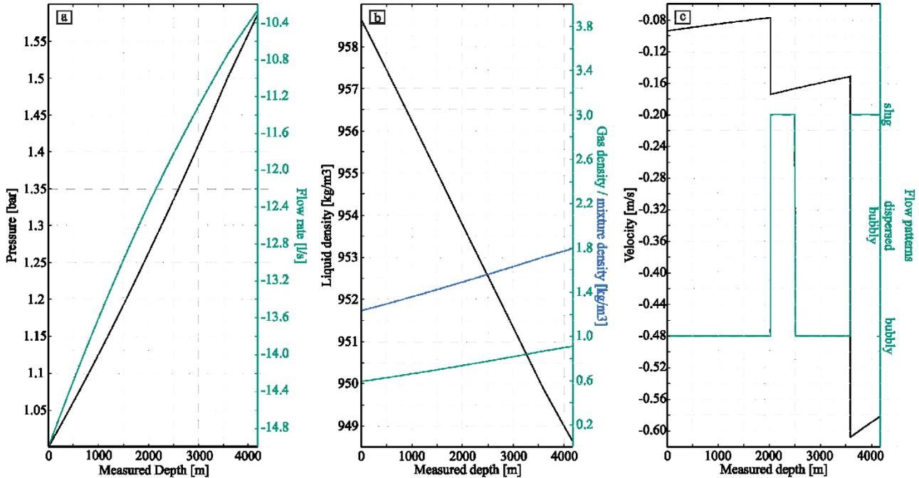
**Figure 4:** The pressure traverse and the flow rate are non-linear functions (Figure 4a), resulting from varying phase densities (Figure 4b) and changing volume ratios of the phases in the mixture. The decreasing pipe diameter causes increasing flow velocities which results in changing flow patterns alternating from bubbly to slug flow (Figure 4c).
