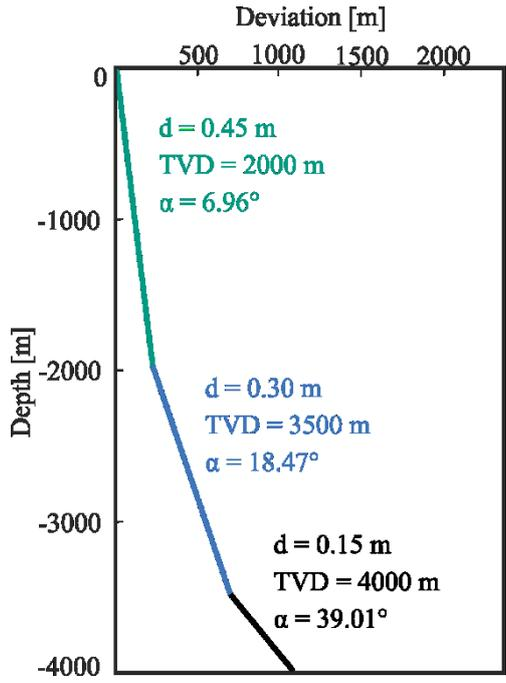
**Figure 3:** Layout of a 4000 m deep (TVD) production well with multiple inclination changes ( $\alpha_1 = 6.96^\circ$ ,  $\alpha_2 = 18.47^\circ$  and  $\alpha_3 = 39.01^\circ$ ) and decreasing diameters ( $d_1 = 0.45$  m,  $d_2 = 0.30$  m and  $d_3 = 0.15$  m).
