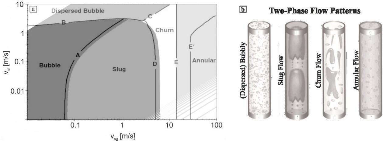
**Figure 2:** a) Validation of two-phase flow patterns. Simulated flow patterns (grey-shaded areas) as functions of superficial gas velocity  $v_{sg}$  and superficial liquid velocity  $v_{sl}$  match experimental data (field boundaries (black lines) according to Ishii and Hibiki, (2006)) in very good agreement. b) Scheme of different flow patterns ((disperse) bubbly, slug flow, churn flow and annular flow), which are evolving as a function of  $v_{sg}$  and  $v_{sl}$ .
