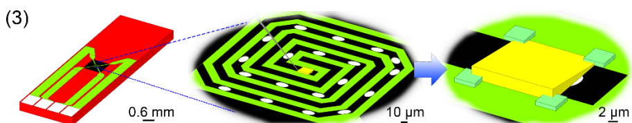
Figure 4.4: Transfer and deposition of the wedge on the MEMS chip (Fam, Sheppard et al. 2019).
