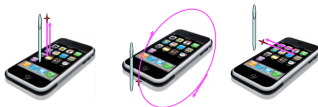
Figure 5.16: Working principle of the MagiSign scheme as depicted in [175] on page 4. The magnet required in the scheme is symbolised by the pen.
