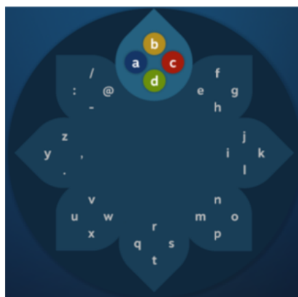
Figure 5.3: The interface of the Daisy Wheel scheme. The upper most petal is selected using the analogue stick. The four characters in the selected petal are coloured reflecting the buttons the users needs to press on the gamepad to enter the respective character.
