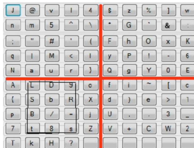
Figure 5.12: Interface of the PairPasswordChar scheme as depicted in [166] on page 167. Illustrated here is the application of the third rule, where the two characters in the password are ‘L’ and ‘s’.
