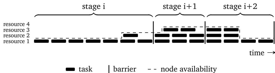
**Figure 2.11:** Exemplary depiction of an elastic micro-task schedule for 3 stages with 8 tasks each.
