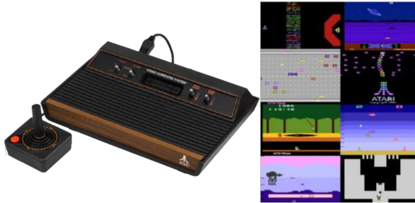
Fig. 7. Left: The Atari 2600 video game console. Right: Screenshots of 8 different Atari games. They show the simple, low resolution graphics of the Atari 2600.
