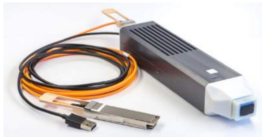
Fig. 10. LightProbe with USB interface for power and control and the optical interface for data[8]
