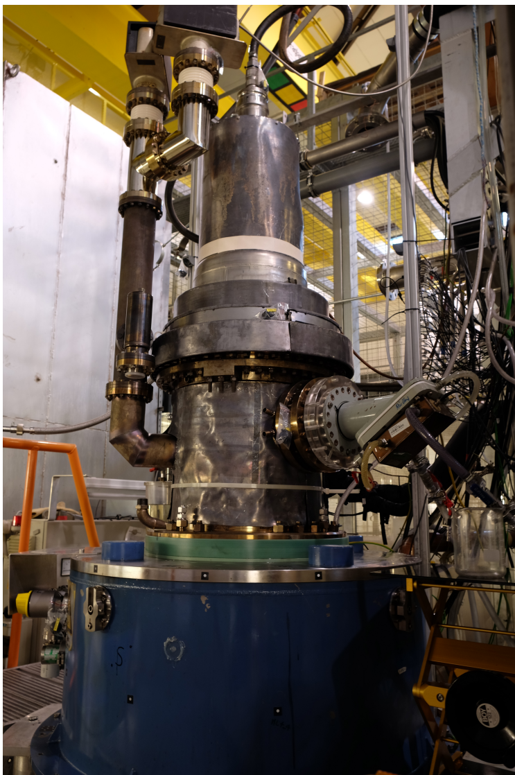
Figure 7.1: The coaxial-cavity pre-prototype long-pulse gyrotron in the superconducting magnet with the calorimeter for the RF power measurement.
