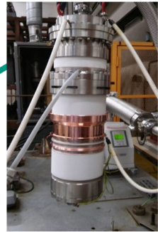
Figure 6.1: Assembled coaxial-cavity long-pulse gyrotron equipped with the old pre-prototype short-pulse Magnetron Injection Gun.
