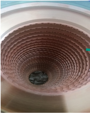
Figure 6.1: Assembled coaxial-cavity long-pulse gyrotron equipped with the old pre-prototype short-pulse Magnetron Injection Gun.
