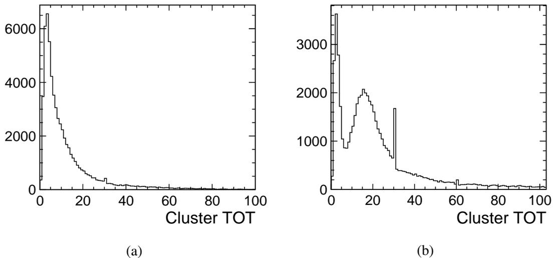
Figure 6.22 Resulting amplitude spectrum from a  $^{90}\text{Sr}$  source, for a capacitively coupled assembly with (a) a 20  $\Omega\text{cm}$  and (b) a 1000  $\Omega\text{cm}$  C3PD sensor. The peaks observed for the ToT value of 30 are resulting from single cluster hits where the ToT counter has saturated.
