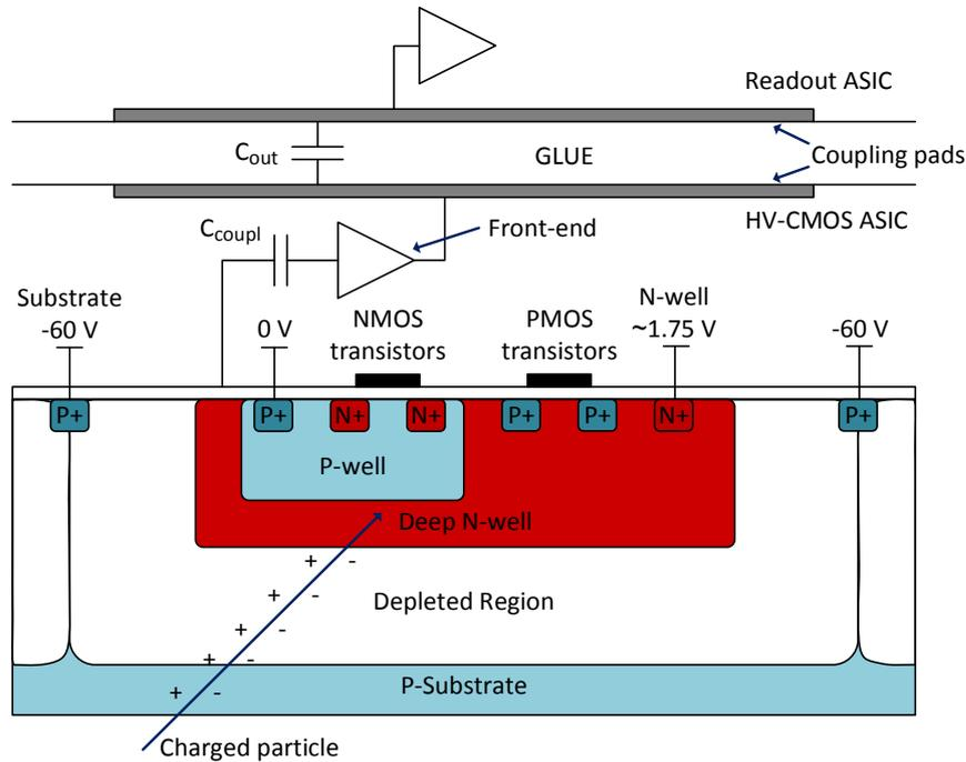
Figure 5.1 Schematic cross-section of a capacitively coupled assembly.
