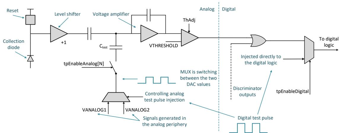
Figure 7.7 Test pulse injection in the CLICTD cell.
