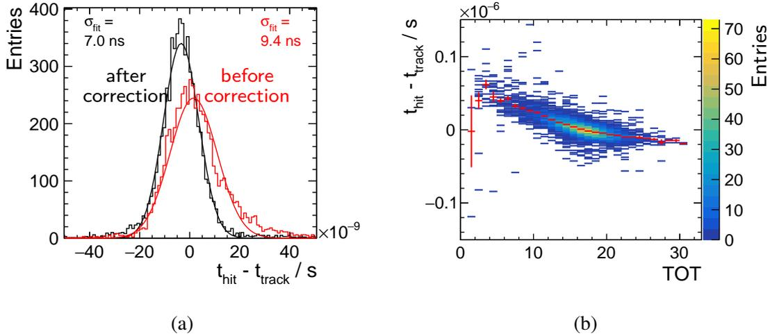
Figure 6.26 (a) Time difference between the reconstructed hit and the track and (b) ToT information used to correct for the time walk effect. From [91].
