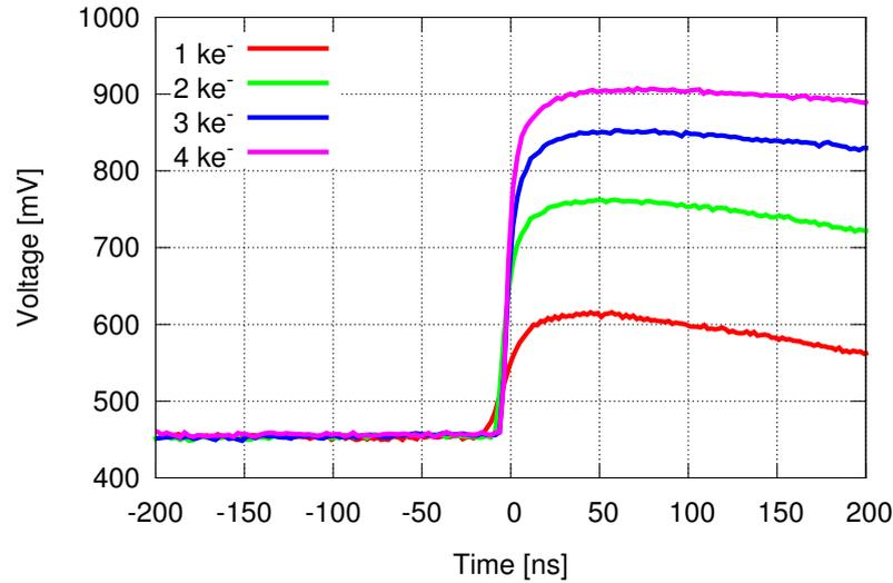
Figure 6.17 Output pulses (averaged over 16 samples) for different charge injected using test pulse. From [74].
