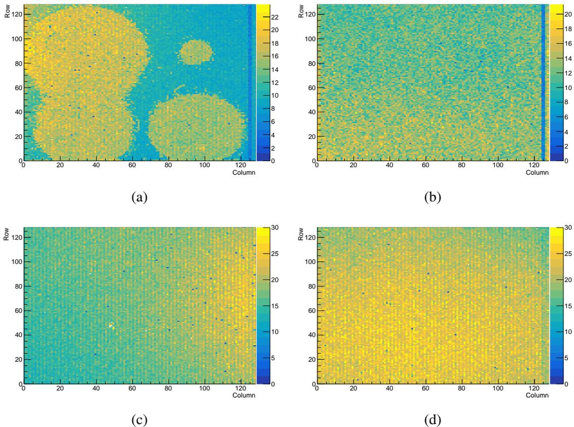
Figure 6.20 Hit maps acquired with the CLICpix2 readout chip, after injecting test pulses in the C3PD front-end. Figures (a) and (b) present two capacitively coupled assemblies with 20  $\Omega$ cm C3PD sensor chips and Figures (c) and (d) present two assemblies with 1 k $\Omega$ cm C3PD chips.
