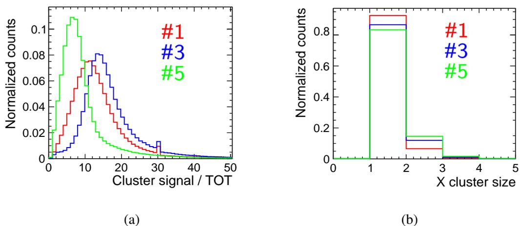
Figure 6.24 (a) Cluster signal and (b) cluster size as measured in beam tests with three different capacitively coupled assemblies. From [91].
