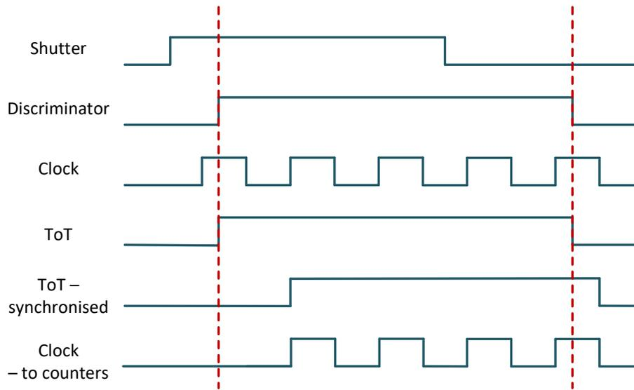
Figure 7.9 ToT measurement in the CLICTD cell.
