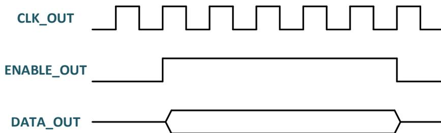
Figure 7.14 Timing diagram of the CLICTD readout.
