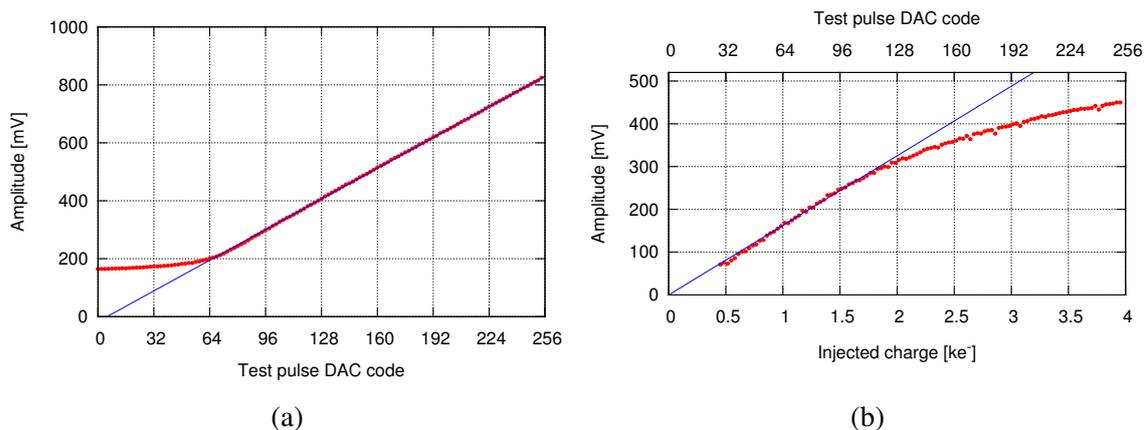
Figure 6.16 (a) Injected test pulse amplitude and (b) output amplitude (averaged over 16 samples) as a function of the test pulse DAC code. From [74].
