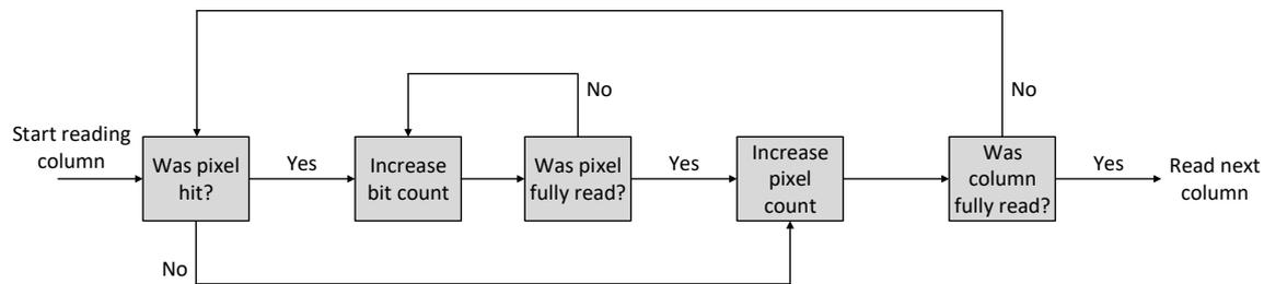
Figure 7.10 Algorithm diagram of the CLICTD End-of-Column block.
