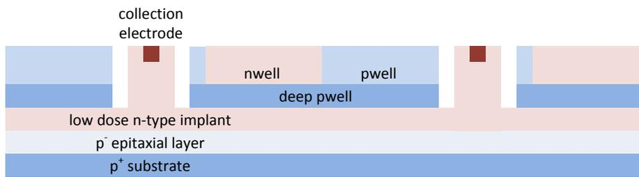
Figure 7.1 Process cross-section - continuous N-implant (not to scale).
