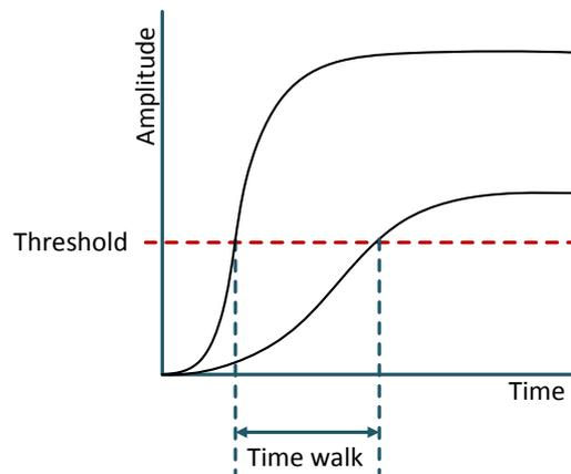
Figure 3.5 Time walk in a detector.
