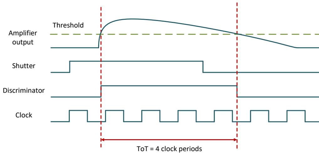
Figure 3.4 Timing diagram of a ToT measurement.
