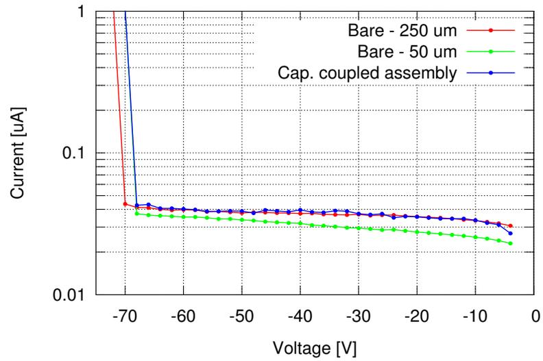
Figure 6.14 I-V curve for a C3PD chip in a capacitively coupled assembly, compared to the I-V curves for two bare chips: one 250 μm thick and one thinned down to 50 μm.
