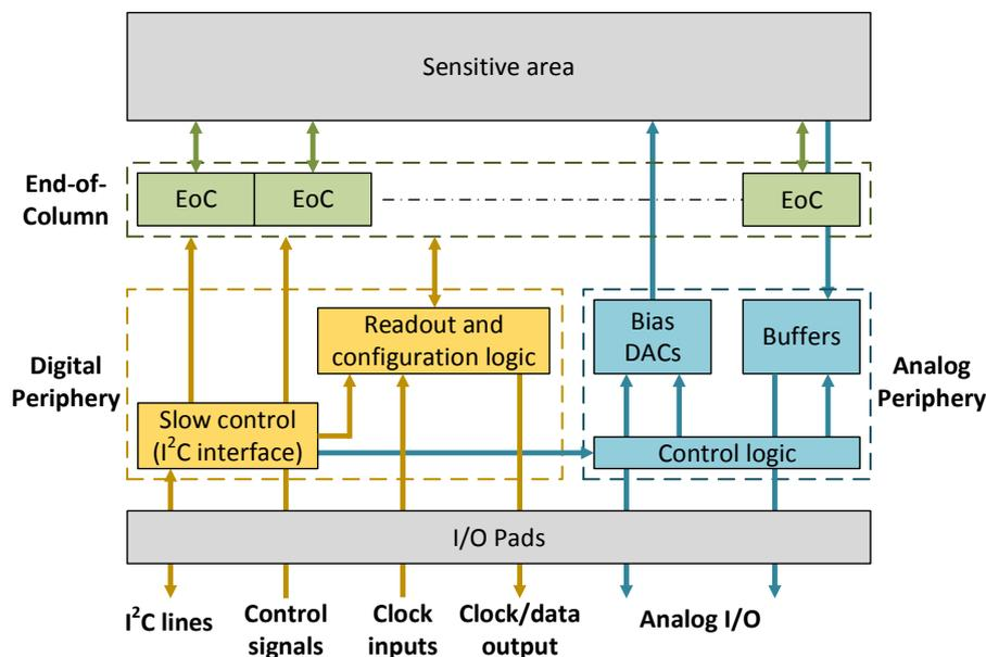
Figure 7.11 Block diagram of the CLICTD periphery.
