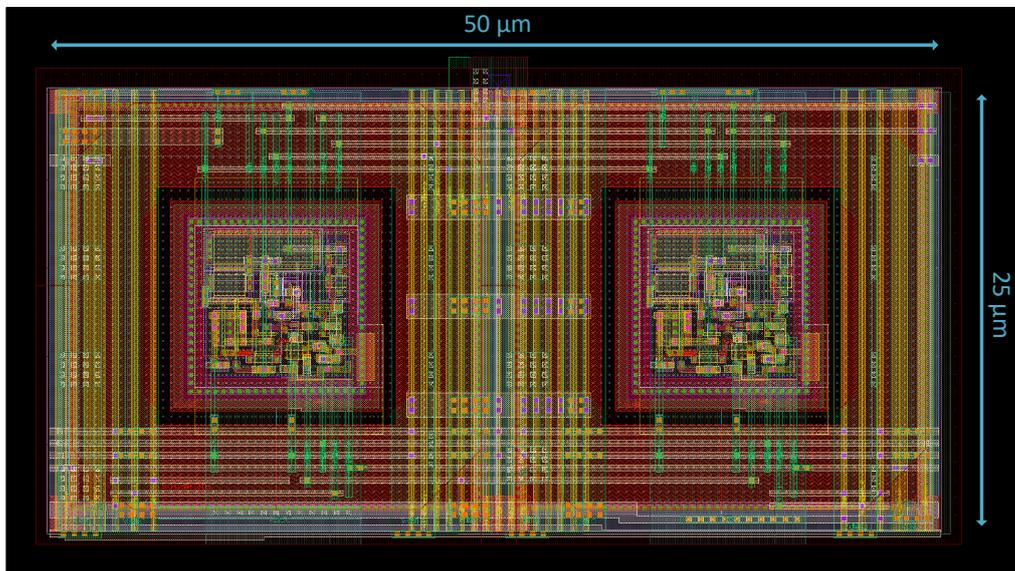
Figure 5.4 C3PD double pixel layout. The pixels are shown to the left and the right side. The biasing lines are routed between the pixels.
