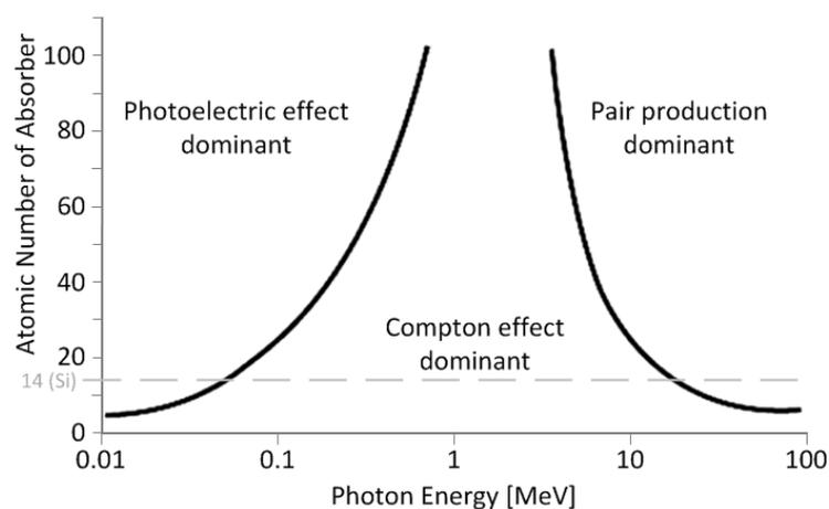
Figure 3.1 Interaction of photons with matter. From [12].
