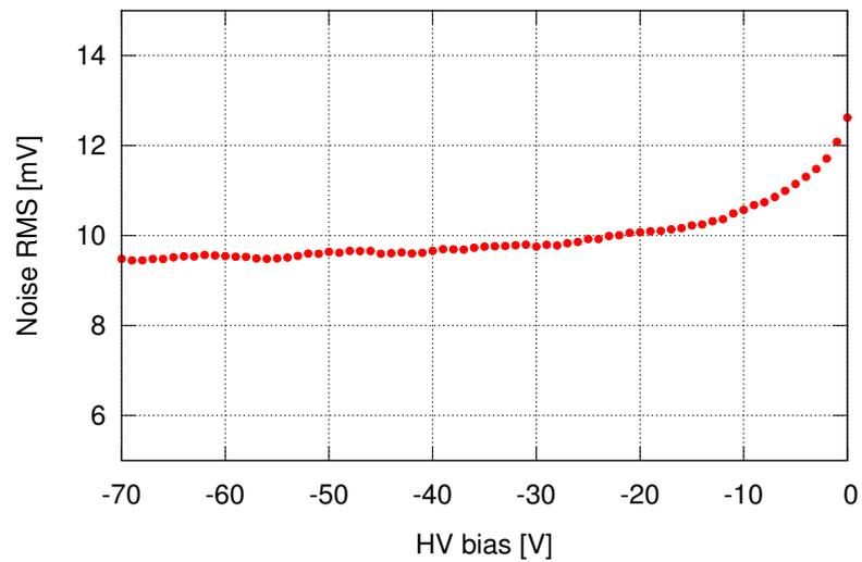
Figure 6.15 Noise at the amplifier output as a function of the high voltage bias. From [74].
