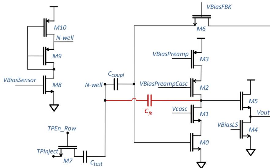
Figure 5.3 C3PD pixel schematic. The parasitic feedback capacitance is shown in red colour.
