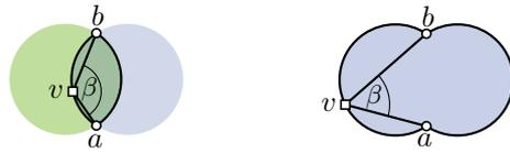
**Figure 6.8:** The angle  $\angle avb$  is at least  $\beta$  for  $\beta > 90^\circ$  ( $\beta < 90^\circ$ ) if and only if  $v$  lies in the intersection (union) of two discs (including its boundary, but excluding  $a$  and  $b$ ).
