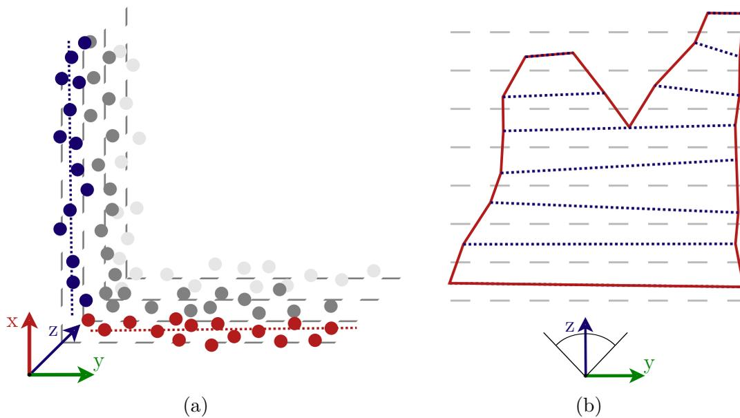
Figure 4.5: We cluster each slice’s points and use RANSAC to detect line segments (a). These are then pruned using their slope, only keeping horizontal segments. Our final agglomeration step, starting with the closest slice, iteratively collects these line segments and connects them into an enclosed section, *i.e.*, the final accessible section detection (b).
