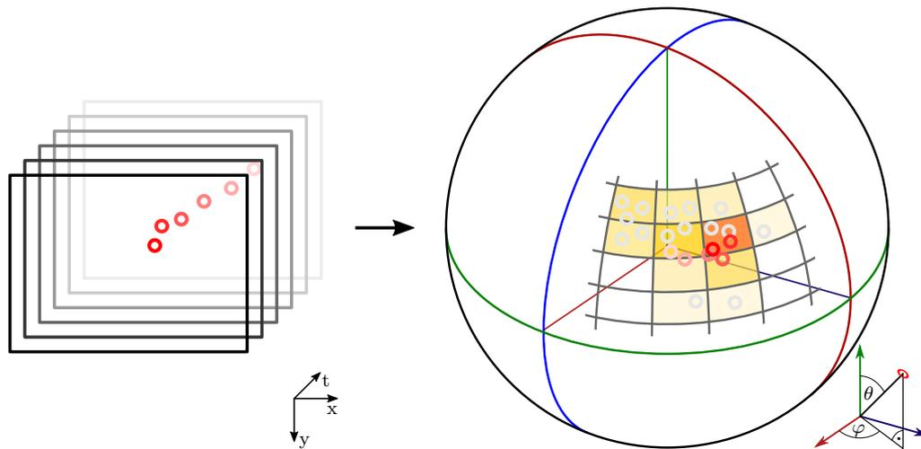
Figure 4.7: We project the frame wise detected vanishing points from image coordinates into spherical coordinates, add these into an accumulator array, and use a frame wise decay to finally report the cell with the maximum value as our tracked vanishing point over time.
