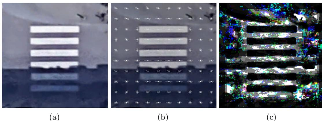
Figure 3.4: Example aerial imagery with (a) a zebra crossing and its feature visualizations: (b) HOG's blockwise computed gradients at a coarse block size for better visibility, and (c) LBPs, where the binary vectors are grouped and visualized by distinct colors, showing the feasibility of these features for this classification task. Aerial imagery © Google Maps.
