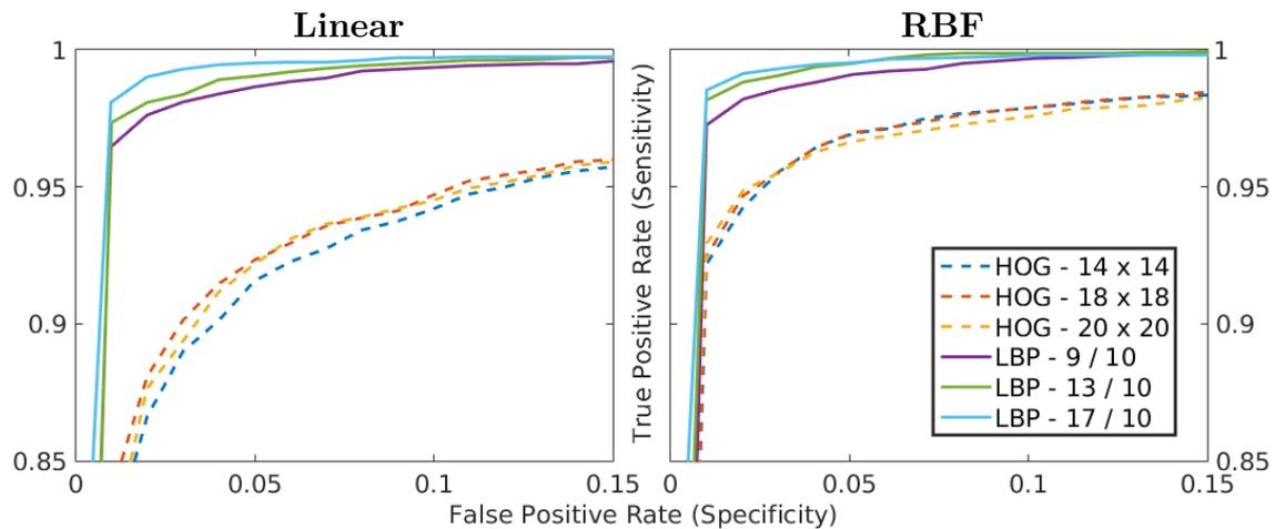
Figure 3.6: Receiver Operating Characteristic (ROC) curves for our zebra crossing detection. We perform a 5-fold cross-validation on our own data, comparing linear kernels, where the HOG feature performs much worse than LBP, and RBF kernels, where the selected feature and its specific parameters make less of a difference.
