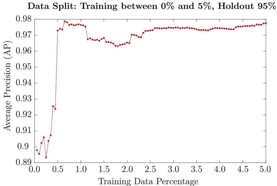
Figure 3.5: Average precision curve for our zebra crossing classification approach when using very little data. We randomly split our dataset ( $\sim 3100$  positive and  $\sim 3100$  negative instances) into a training and a holdout test split. We then train SVMs using between 0% and 5% of all available data, increasing the amount of used data in steps of 0.05%.
