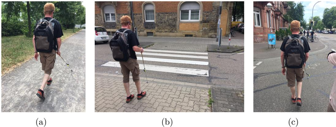
Figure 5.3: A participant during the **TERRAIN** user study: (a) on a pedestrian walkway, (b) in front of a zebra crossing, (c) crossing at a pedestrian traffic light. The backpack contains the prototype’s processing unit, while the camera is mounted onto its front strap.
