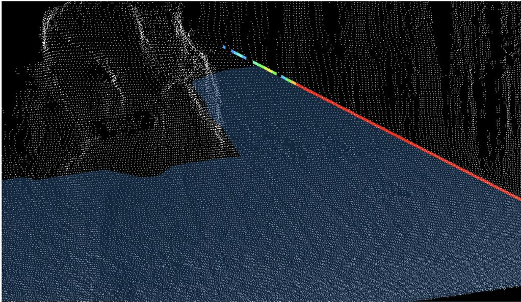
Figure 4.2: Accessible section detection example. Right of the accessible section (blue) is a building’s facade, while the blob on the left is a parked car. Also shown is a detected shoreline (Section 4.2), as both approaches rely on depth data and share the same techniques.
