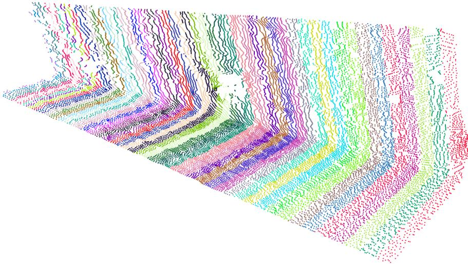
Figure 4.4: Real world data, sliced and color coded. Please note how the noise level increases significantly for very far away slices. Also, when setting all slices to a constant width, the number of points per slice decreases for further away slices due to optical constraints.
