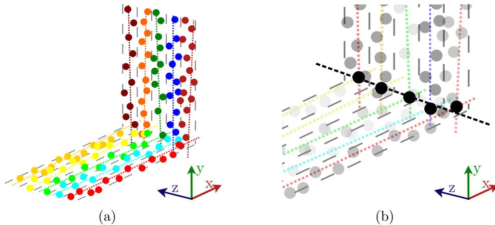
Figure 4.8: Our Slice&Dice-based clustering (*cf.* Section 4.1.2). We cluster points slice-wise according to their surface normals, use a weighted RANSAC to detect almost horizontal as well as sufficiently differing line segments, and determine their 2D-intersections in the slice’s main plane (a). We then generate a shoreline candidate from these intersections (b).
