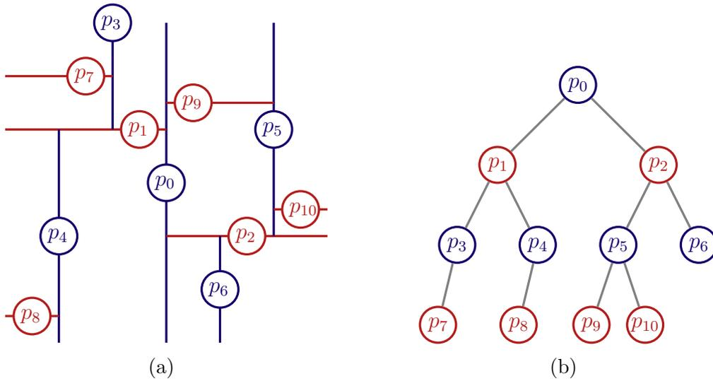
Figure 3.11: A two-dimensional space partitioning  $k$ -d tree (a) of example points and its binary  $k$ -d tree (b) that allows for very efficient range searches in a large sets of points.
