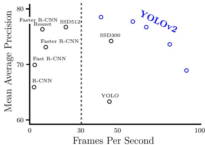
Figure 4.11: YOLO’s speed *vs.* detection precision on the VOC challenge. YOLOv2 provides a great speedup when compared to other available deep learning architectures and even YOLOv1. © Redmon and Farhadi
