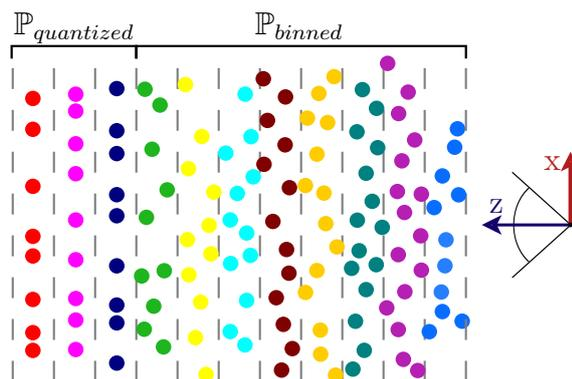
Figure 4.3: Our proposed Slice&Dice approach separates depth data into individual depth slices, based on each point’s  $z$ -value, *i.e.*, its distance to the camera (colored point groups). For further processing, these can be either quantized ( $\mathbb{P}_{quantized}$ ), mapping the points onto a plane, or left unchanged ( $\mathbb{P}_{binned}$ ), if a binning approach is preferred to not lose any depth information, largely depending on further processing steps and required depth precision.
