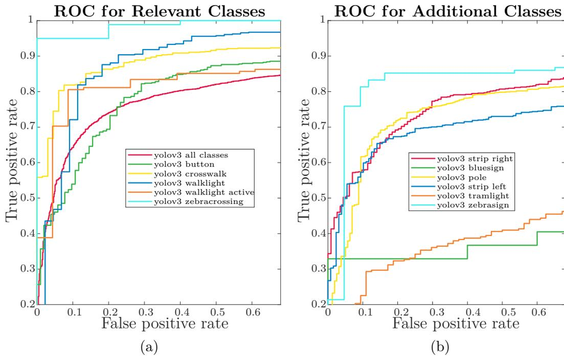
Figure 4.13: ROC results for relevant pedestrian crossing classes (a) as well as additional ones (b). All relevant classes are detected with high accuracy, while decreased accuracy for other classes is mostly due to them being underrepresented in our training data.
