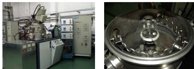
Fig. 4. Balzers system facility: a) general view, b) position of flat, circular magnetrons, c) chamber overview
