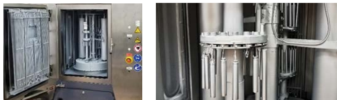
Fig. 3. Images of the Hauser Flexicoat 850 at CTU in Prague. Deposition chamber (left); Rotating sample holders with Cr target in the back (right).
