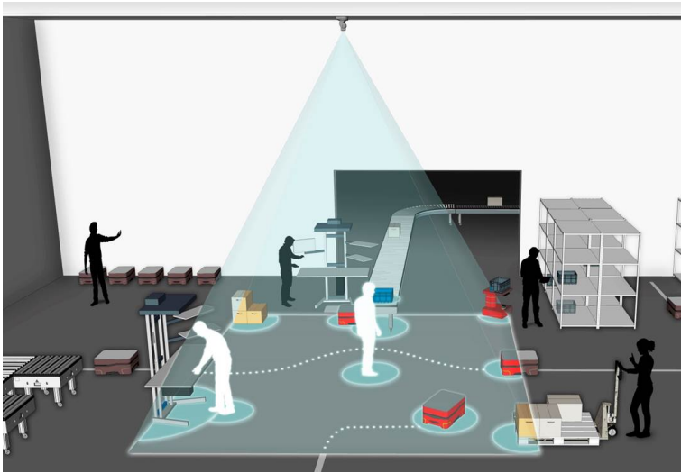
Abbildung 0.2: Schematic representation of the sensor unit including the monitored area in which the driverless transport vehicles can navigate freely.
