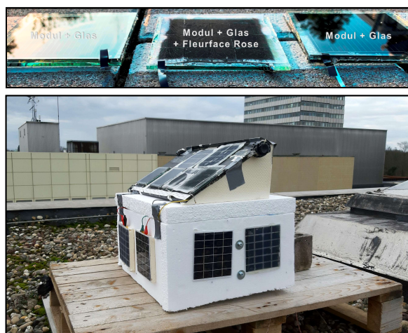
Outdoor performance monitoring under various module orientations.
