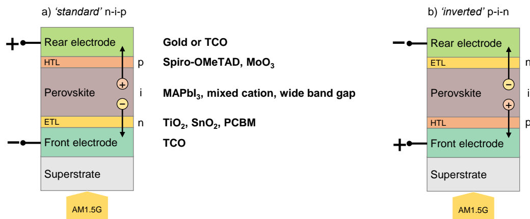
Figure 2.3: Different architectures of perovskite solar cells in a) standard and b) inverted architecture.
