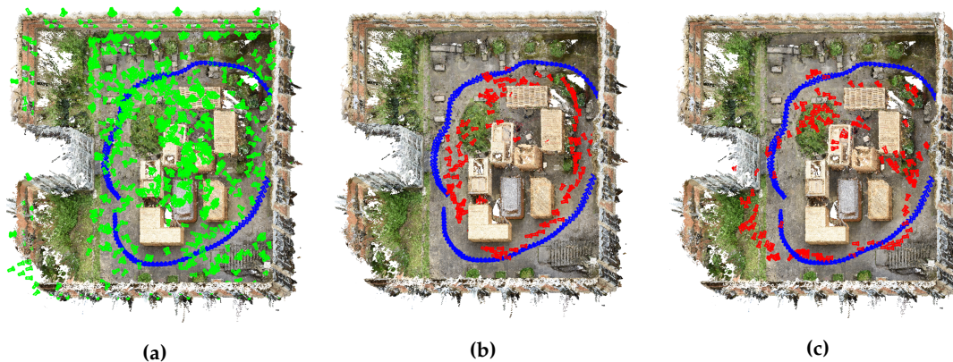
Figure 8.1: Medium coverage set . Training poses (green), evaluation poses (blue) and estimated poses (red). Visualization of (a) training poses and evaluation poses, (b) pose estimates derived by the modified VGG16-Net and (c) pose estimates derived by SqueezePoseNet.
