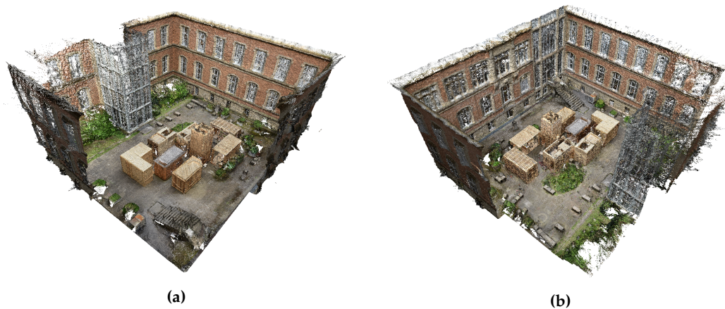
Figure 4.1: Side views of the reconstructed 3D model of the atrium. The red bricked walls show very similar structures, leading to a challenging scene for computer vision algorithms.
