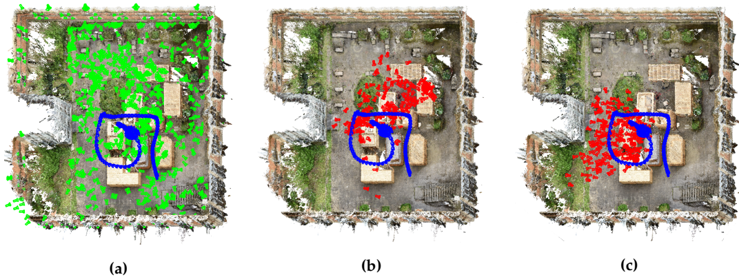
Figure 8.3: Low coverage set . Training poses (green), evaluation poses (blue) and estimated poses (red). Visualization of (a) training poses and evaluation poses, (b) pose estimates derived by the modified VGG16-Net and (c) pose estimates derived by SqueezePoseNet.
