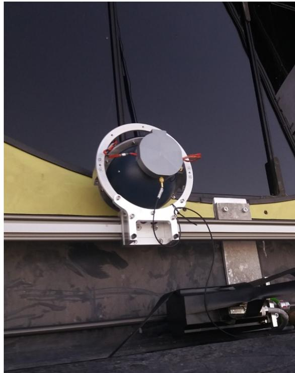
**Figure B.4:** Photo of an alternative design for the sphere holding structure meant to correct for imprecision in the first prototype. It was only used in few measurements in the field and then dropped in favor of the holding structure of the Czech sphere.
