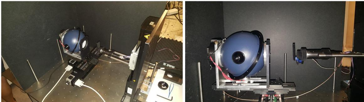
**Figure 4.6:** Test stand in Olomouc. The horizontal linear stage and the rotational stage is in the foot for the sphere. The vertical linear stage is attached to the detector, which consists of a SiPM behind a double pinhole. The second rotation is done by rotating the sphere in its mount. [95]
