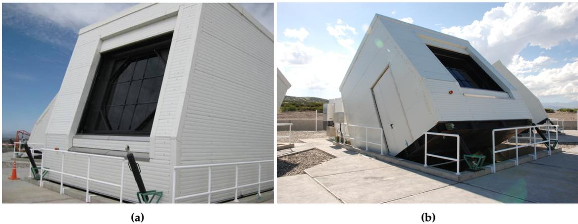
Figure 2.14: The HEAT telescopes in (a) downward and (b) upward mode [36].
