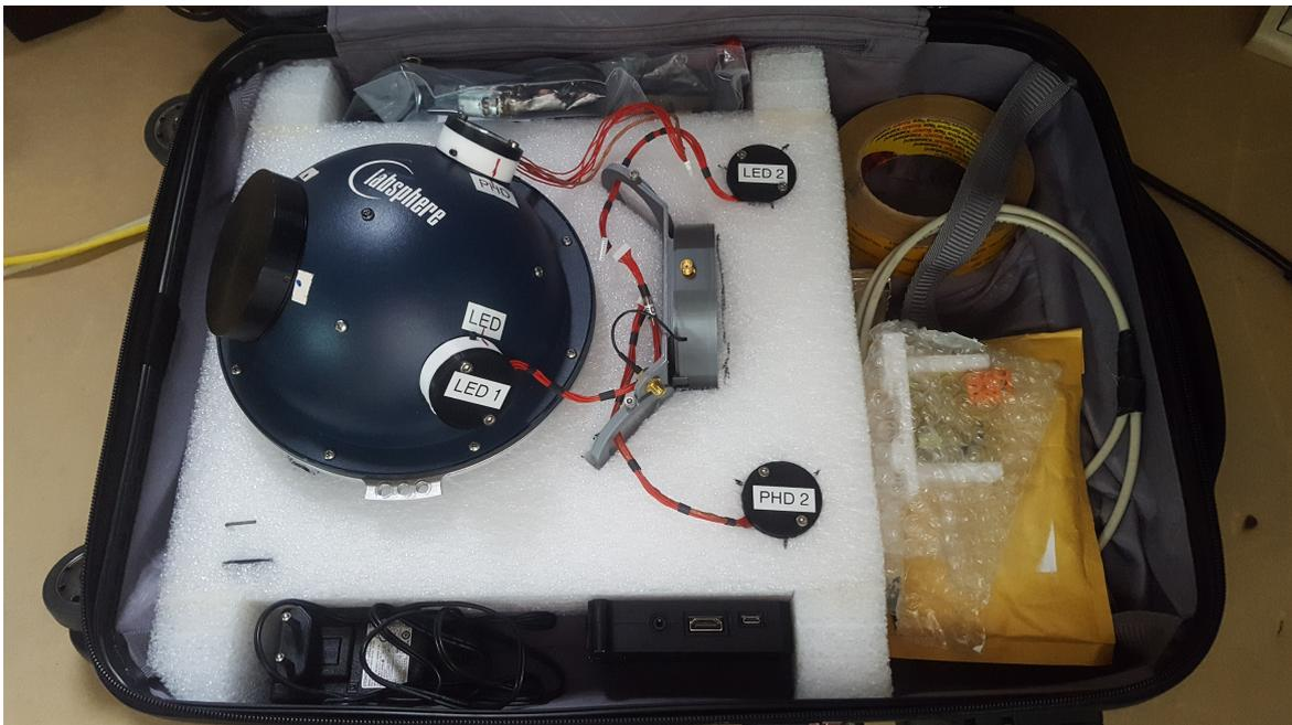
**Figure B.5:** Transport case of the Karlsruhe sphere, can be brought as hand luggage on flights.
