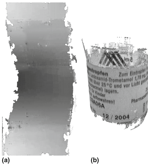
Fig. 14 a Subpixel-precise disparity image of the rectified image of Fig. 13a. b 3D stereo reconstruction with texture mapping
