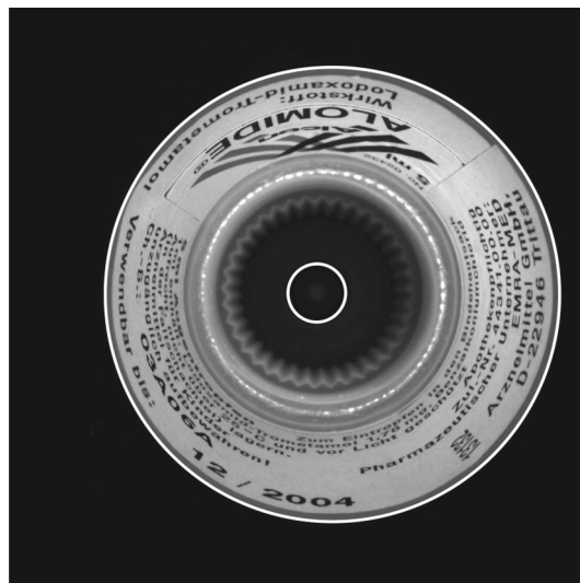
Fig. 15 Two extracted ellipses (white) of the circular ground plane (large ellipse) and the circular screw cap (small ellipse) of the bottle that are used to determine the pose of the cylindrical surface of the text label
