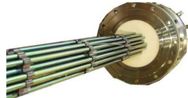
QUENCH bundle for large-scale experiments
