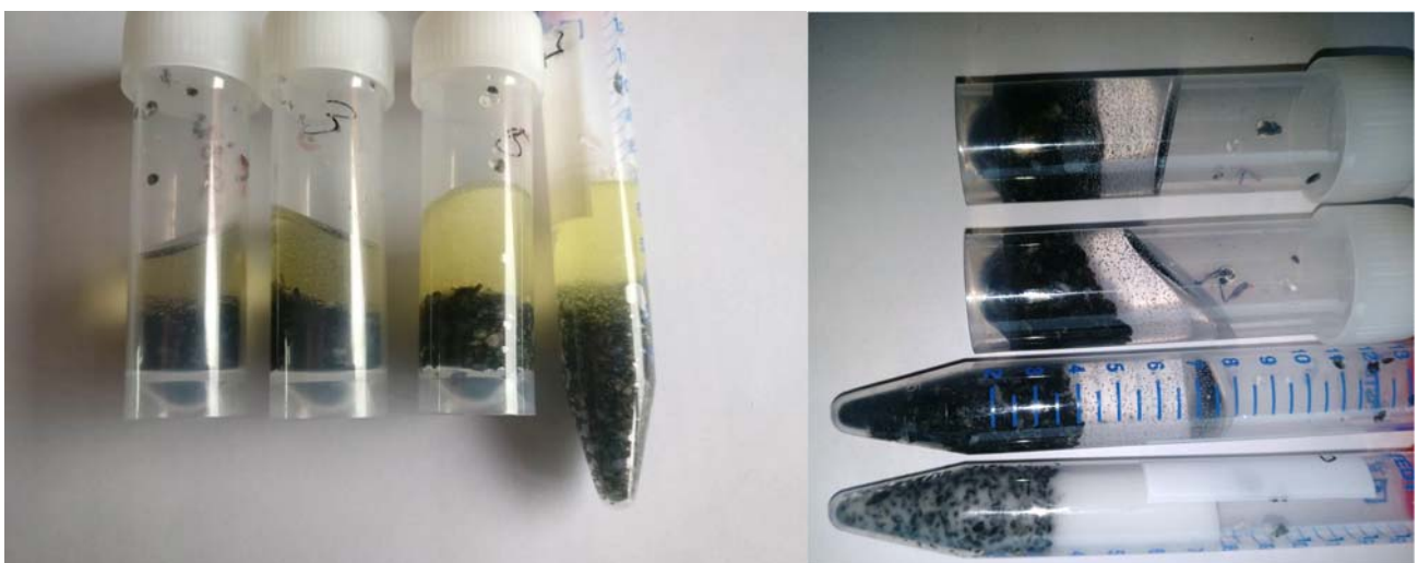
Figure 21: FFM Resin impregnation after washing with 90/10, 80/20, 70/30, 50/50% MeOH/GGW mixture (from left to right). Sika-52 samples are shown in the left and Araldite samples in the right picture
