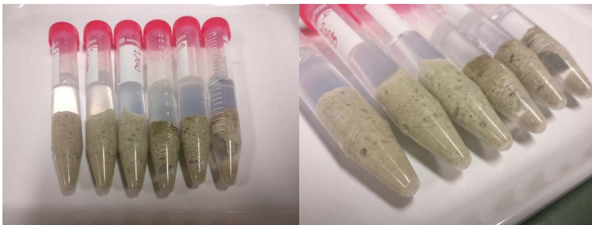
Figure 23: Araldite impregnated Febex samples: #2, 4, 6, 8, 10, 12 from left to right
