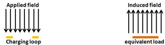
(b) Equivalent 2D  $H$ -formulation FEM model for HTS flux pump
