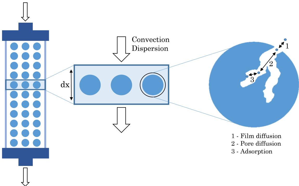
*Figure 1.4: Processes in chromatographic columns, which can be modeled by setting up differential mass balances. Not included in the figure is surface diffusion, which can also contribute to mass transfer inside the pores. Figure adapted from Seidel-Morgenstern et al.<sup>94</sup>.*
