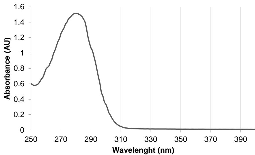
*Suppl. Figure 3:* Pure component UV/Vis absorbance spectrum of 5T4 mAb measured in Tecan plate reader M200 Pro at a concentration of 2 mg/mL (in 50 mM sodium phosphate buffer).
