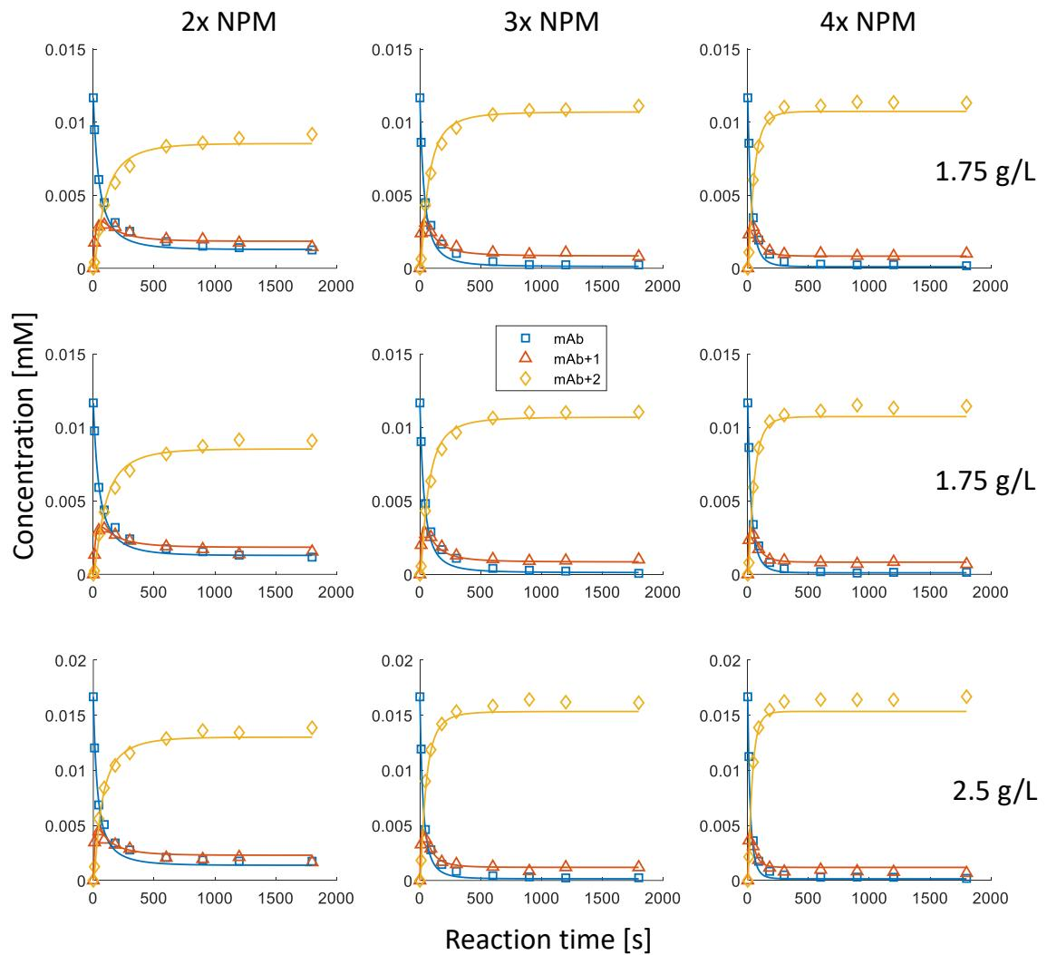
*Figure 5.5: Results of model 5 prediction for the 9 validation experiments. The markers are experimental data and the respective model predictions are shown by straight lines. The blue square markers are the un-conjugated mAb, the red triangles the mono-conjugated mAb, and the yellow diamonds the bi-conjugated mAb.  $R^2$  of prediction was at 0.978 and RMSEP at 0.00070 mM. The data at 2.5 g/L is outside the calibration range of the model (1-2 g/L).*
