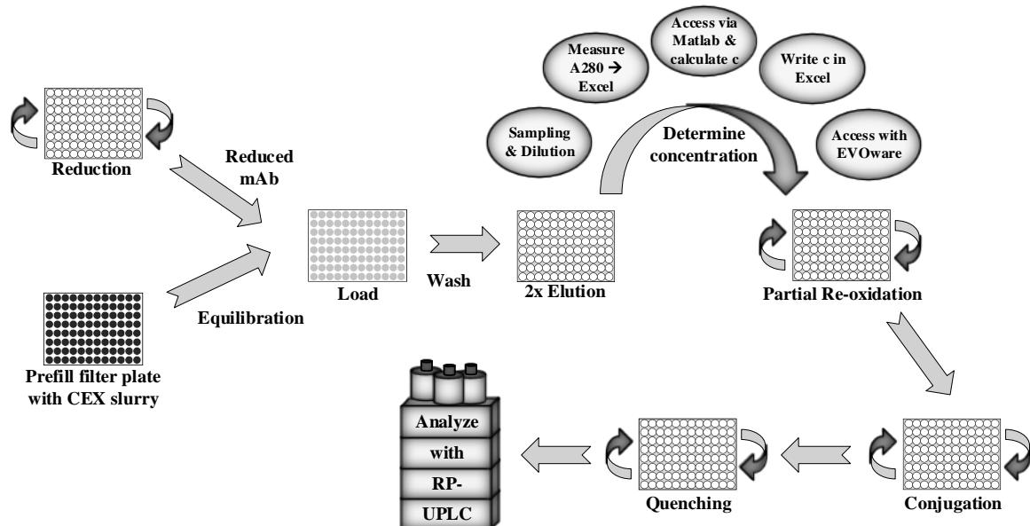
Figure 3.2: High-throughput platform for conjugation process development on automated liquid handling station. The concentration  $c$  stands for the mAb concentration after the buffer exchange step, which is determined to calculate reagent concentrations for the following steps.
