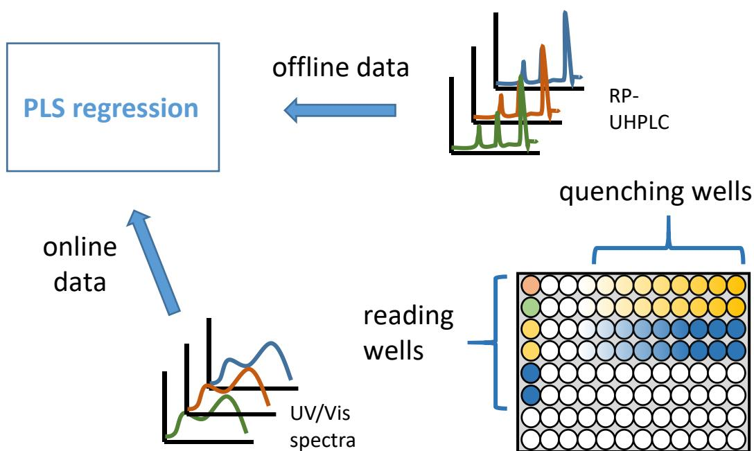
*Figure 4.2: Experimental setup used for high-throughput on-line monitoring in microplate format. UV/Vis spectra were recorded during the conjugation reaction using the integrated Tecan plate reader. Reactions in the quenching wells were stopped at different time points and analyzed by RP-UHPLC. On-line and off-line data was used for the generation of PLS regression models.*
