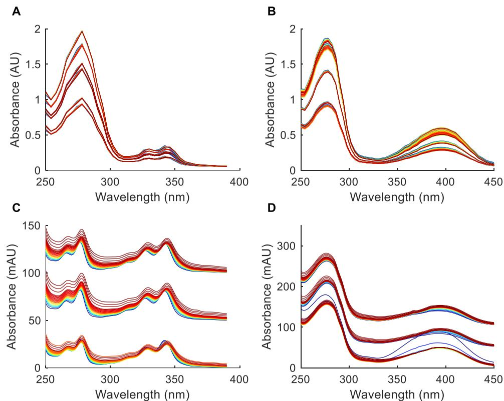
*Suppl. Figure 1: Raw spectra of all calibration samples. The spectra are colored according to the reaction progress from blue to red. The microplate experiments are depicted in the top row, while the bottom row shows the spectra recorded in the lab-scale setup. Since the lab-scale experiments were performed at the same nominal mAb concentration, the different runs are artificially offset by 50 mAU. The left column shows experiments with NPM, the right column shows experiments with CPM.*
