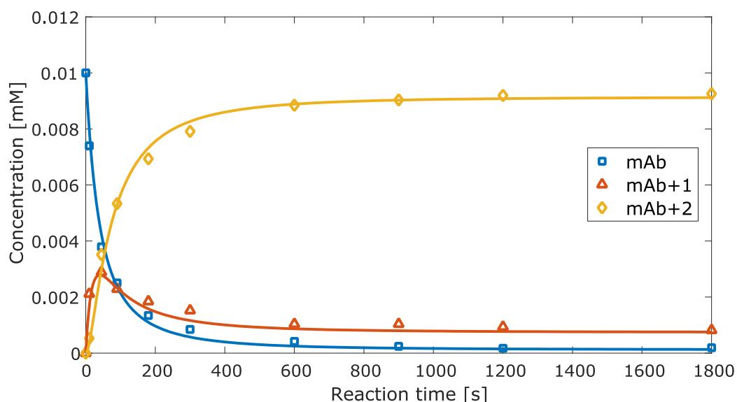
Figure 5.4: Example of conjugation run from the calibration set at 1.5 g/L and NPM ratio of 3. The markers are experimental data, the straight lines the fit for model 5. The blue square markers are the un-conjugated mAb, the red triangles the mono-conjugated mAb, and the yellow diamonds the bi-conjugated mAb.
