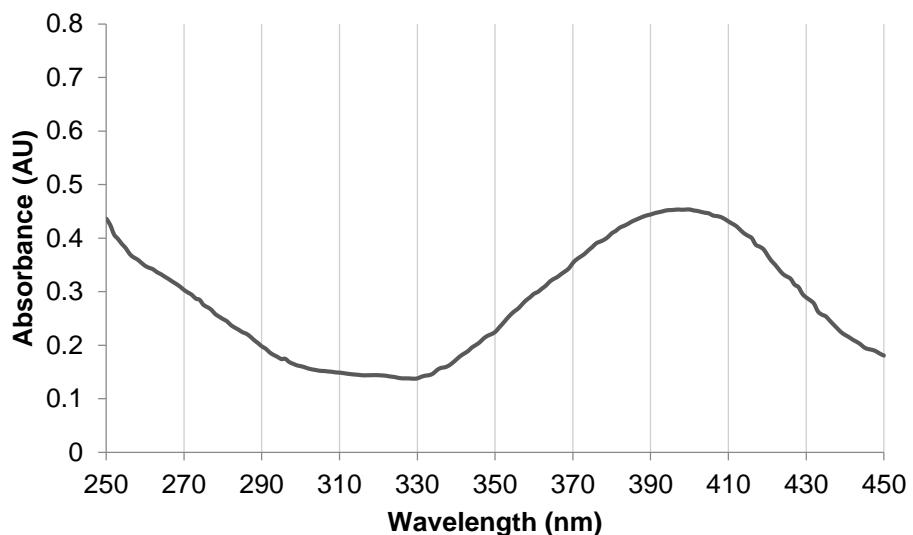
*Suppl. Figure 5: Pure component UV/Vis absorbance spectrum of CPM in phosphate buffer containing 10% of DMSO measured in Tecan plate reader M200 Pro.*
