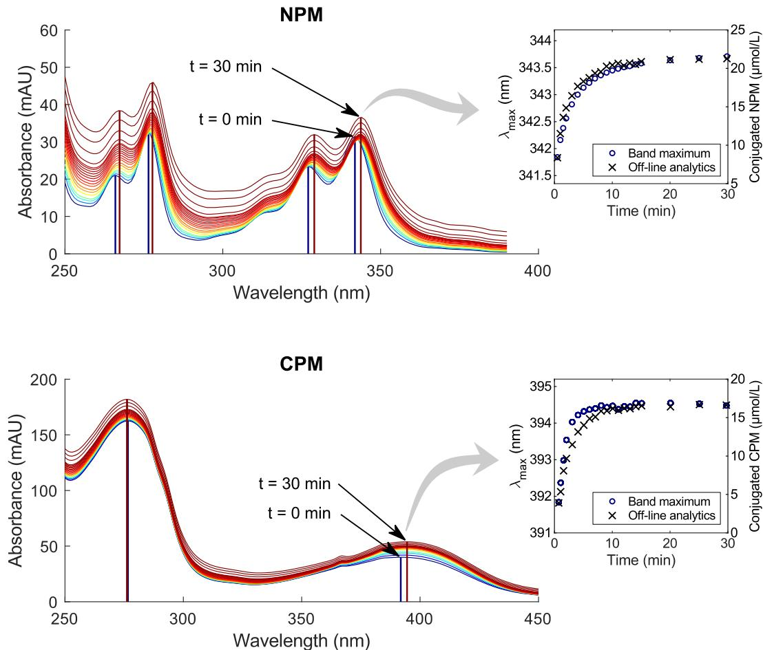
*Figure 4.3: The raw spectra of two lab-scale experiments for NPM (top) and CPM (bottom) are shown. The spectra are colored according to the reaction progress from blue to red. The location of the band maxima of the first (0 min) and the last spectrum (30 min) are marked by vertical lines. On the right side, the time evolution of the band maxima location is compared to the amount of conjugated drug measured by off-line analytics.*
