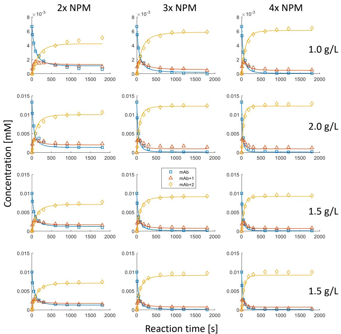
*Suppl. Figure 6: Results of model 5 calibration for the 12 calibration experiments. Markers are experimental data and the respective model predictions are shown by straight lines. Blue square markers are the un-conjugated mAb, red triangles the mono-conjugated mAb and yellow diamonds the bi-conjugated mAb.  $R^2$  was at 0.970.*
