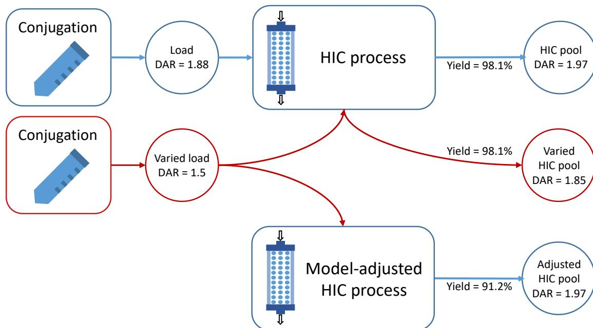
Figure 6.5: This flow chart shows how a mechanistic chromatography model can be applied for more robustly achieving the specified degree of conjugation in the pool. By adjusting the process using the model, one can react to a variation in a previous process step, here the conjugation reaction.
