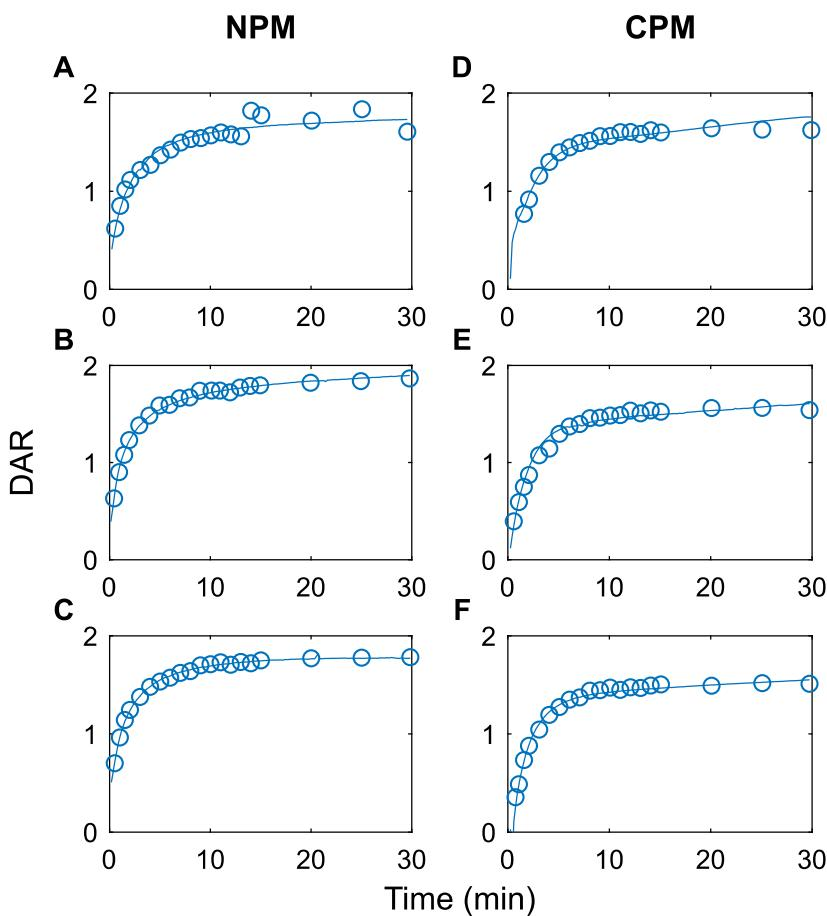
*Figure 4.6: PLS model calibration for the lab-scale experiments is shown for NPM (A, B, C) and CPM (D, E, F). Each model was calibrated on 3 replicates shown in the different subplots. The DAR was used for plotting as it is frequently used to specify the conjugation degree of ADCs. For calculating the DAR, a constant protein concentration was assumed over the course of the reaction.*
