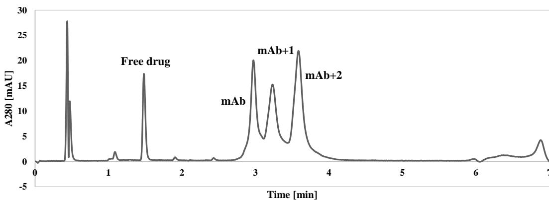
*Figure 3.4: Reversed-phase chromatogram of the analytical separation of unconjugated, mono-conjugated, di-conjugated antibodies and residual free CPM. This example was taken from the comparability study. The starting concentration was 2 mg/mL and the conjugation was stopped after 45 s.*
