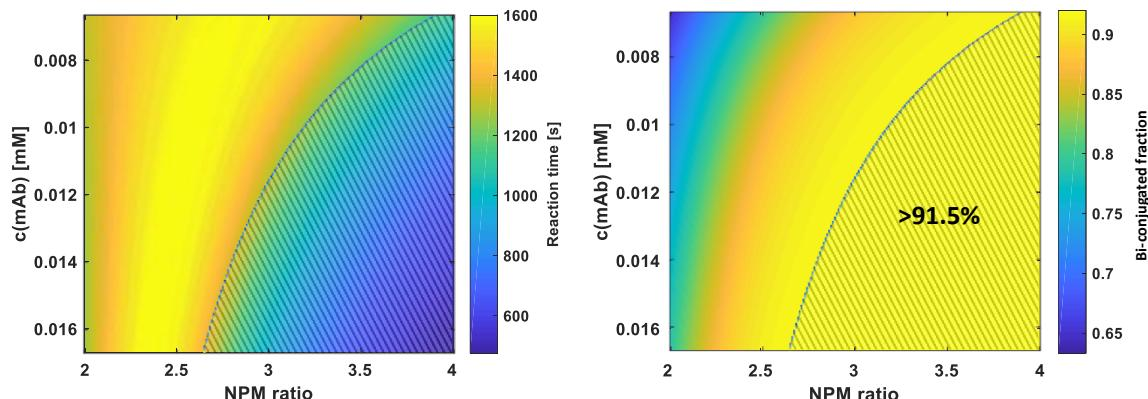
*Figure 5.7: Results of in silico screening and optimization. Color maps show optimal reaction times (left) for screened mAb and NPM concentrations and the resulting fraction of bi-conjugated component (right). The shaded area in both graphs indicates a bi-conjugated fraction of greater than 91.5%.*
