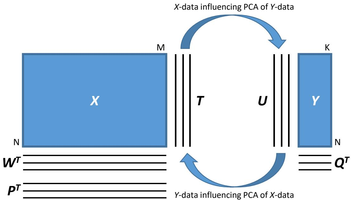
*Figure 1.3: Principle of PLS regression. A PCA is performed for predictor data  $X$  as well as response data  $Y$ . These two PCAs influence each other, resulting in a regression model for the response.  $T$  and  $P^T$  are the scores and loadings matrix for  $X$ , respectively, while  $W^T$  are the weighted loadings for  $X$ .  $U$  functions as the scores and  $Q^T$  as the loadings matrix of  $Y$ . Figure adapted from Kessler<sup>78</sup>.*
