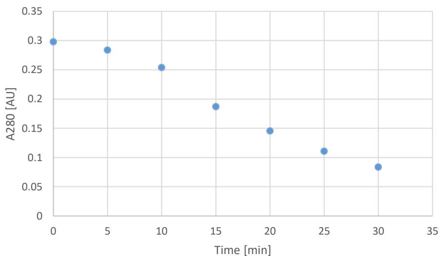
Suppl. Figure 7: Absorption at 280 nm over time measured in Tecan plate reader for a 0.04 mM NPM solution in 50 mM sodium phosphate buffer containing 10% DMSO. The solution was held in a shaken 2 mL Eppendorf Safelock Tube and 200 µL samples were taken every 5 min and measured in a Greiner UV-star microplate.
