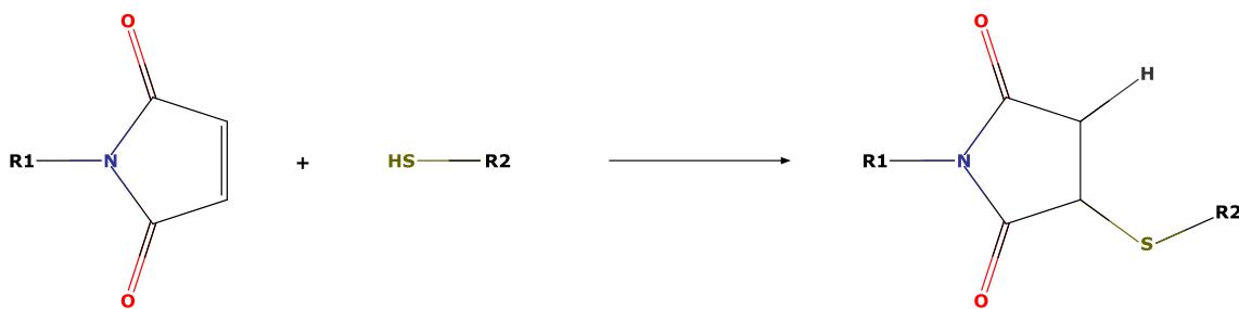
*Figure 3.1: Reaction scheme for the conjugation reaction. The maleimide functionality of the CPM molecule reacts with the thiol group of the two engineered cysteine residues of the antibody, forming a stable thioether bond.*
