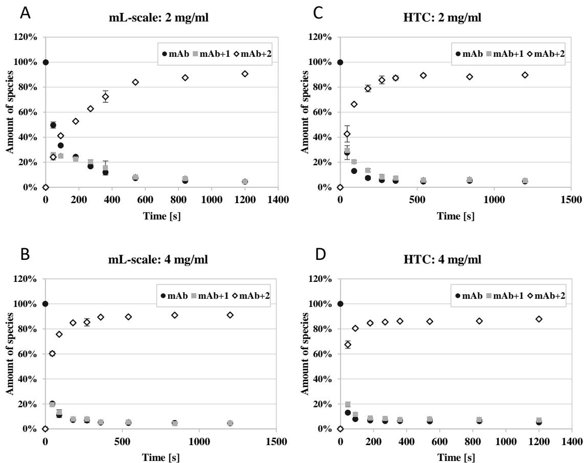
*Figure 3.6: Comparability study with 2 and 4 mg/mL starting antibody concentration. Comparison of reactions in mL-scale process (A, B) and 200  $\mu$ L-scale automated high-throughput process (C, D). The amount of each conjugate species (unconjugated, mono-conjugated, di-conjugated) is depicted as a function of reaction time.*
