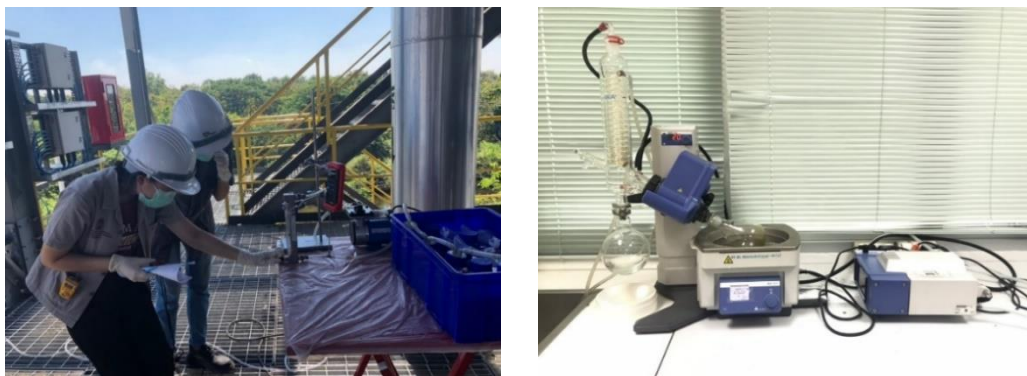
Figure 6. Tar sampling at Nongbua power plant and tar evaporation in the lab at KMITL.
