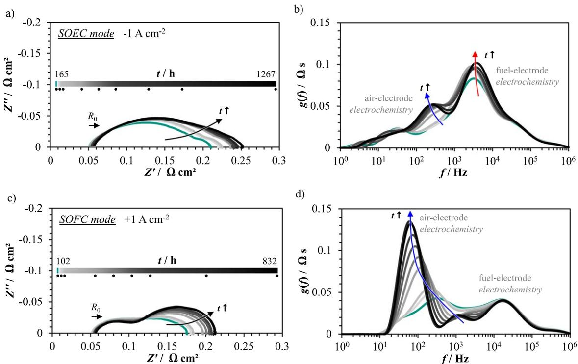
**Figure 7.** Series of impedance spectra under (a) SOEC and (c) SOFC operation with  $\pm 1 \text{ A cm}^{-2}$  at  $750 \text{ }^\circ\text{C}$ . All impedance spectra were measured under load. (b) and (d) show the corresponding DRT spectra.
