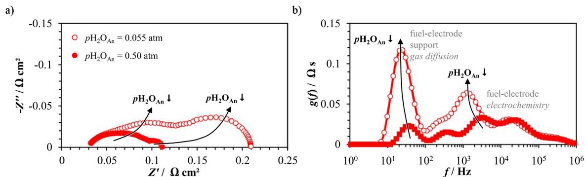
**Figure 3.** (a) Measured impedance spectra and (b) the calculated DRTs for 5.5% and 50% humidified hydrogen as fuel (corresponding to the CV-curves in Fig. 2b). The measurements were performed at 800 °C, under OCV conditions.
