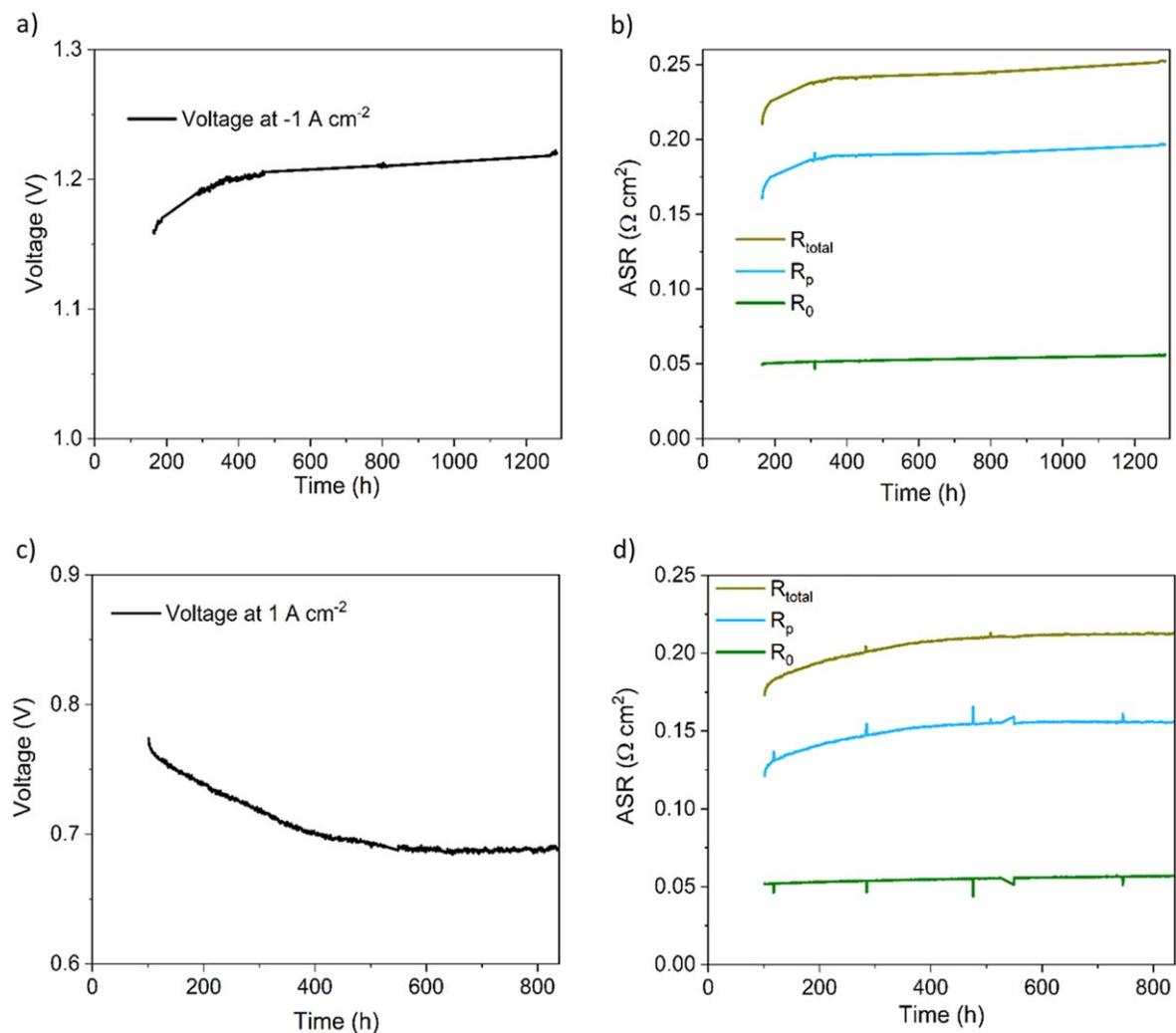
**Figure 6.** Mid-term stability of SOC-KIT at 750 °C under 50%  $\text{H}_2\text{O}$ –50%  $\text{H}_2$  as fuel gas. (a) Voltage degradation at  $-1.0 \text{ A cm}^{-2}$  of a SOC-KIT in SOEC mode. (b) Correlated ASR degradation of the cell in Fig. 6a. (c) Voltage degradation at  $1.0 \text{ A cm}^{-2}$  of a SOC-KIT in SOFC mode. (d) Correlated ASR degradation of the cell in Fig. 6c.
