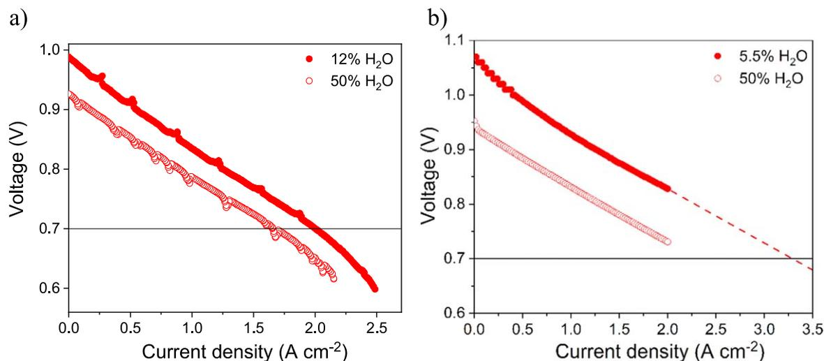
**Figure 2.** Current–voltage investigations of (a) SOC-IEK9 and (b) SOC-KIT at  $800^\circ\text{C}$  in SOFC mode with different  $\text{H}_2\text{O}$  content in  $\text{H}_2\text{O}$ – $\text{H}_2$  fuel gases.
