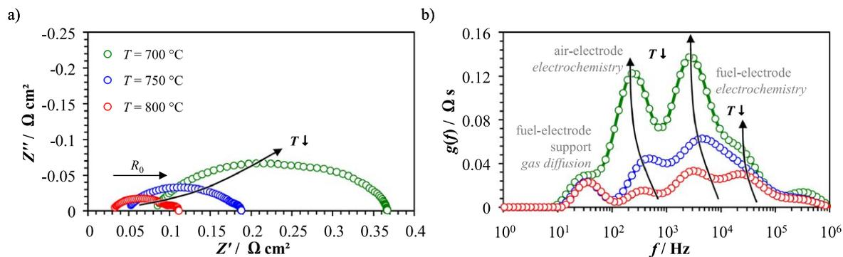
**Figure 5.** (a) Measured impedance spectra and (b) calculated DRTs for varied temperatures between 700 °C and 800 °C (corresponding to the CV curves in Fig. 4). The measurements were performed under OCV conditions with 50% humidified hydrogen as fuel.
