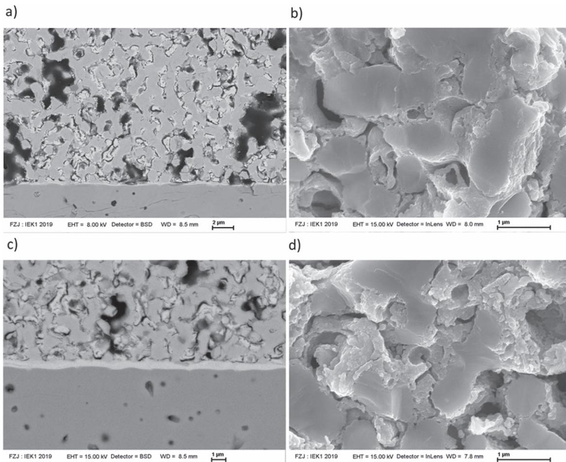
**Figure 9.** Microstructure of LNC97 based air-electrodes. (a) Polished cross-section after short-term operation of 60 h. (b) Fracture after short-term operation of 60 h. (c) Polished cross-section after mid-term operation of 1200 h. (d) Fracture after mid-term operation of 1200 h.
