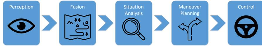
Figure 1.3: Modules of autonomous driving platforms: First the perception based on different sensor types, followed by the fusion of the perceived information to generate a holistic environmental representation. Afterwards, the situation analysis as a base for the maneuver planning. Finally, the execution of the maneuver over the vehicle control system. *Icons are designed by monkik and Freepik from Flaticon.*
