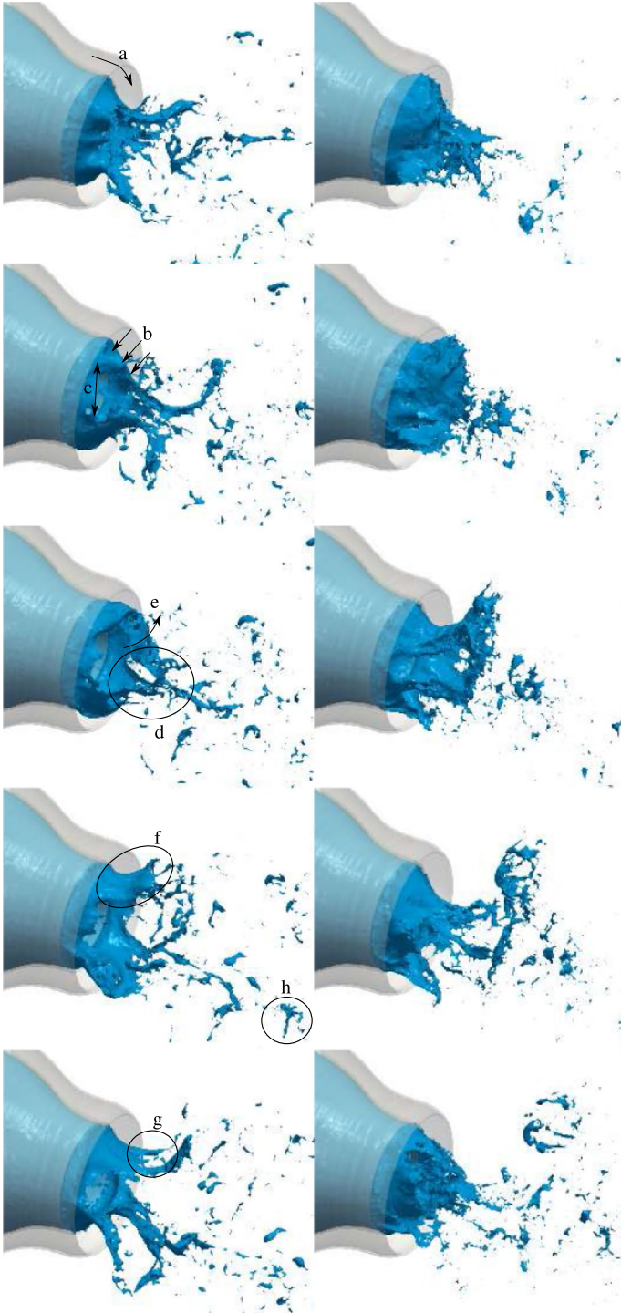
Fig. 11 Time series of a breakup event for L_1 (left, \Delta t = 71.6 \mu\text{s} ) and L_2 (right, \Delta t = 28.2 \mu\text{s} )
