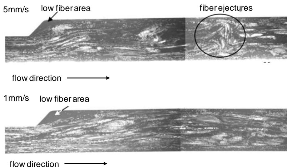
Figure 12: Influence of closing speed on fiber filling at the transition from thin-walled to thick-walled areas adapted from Schmachtenberg et al. (2005)
