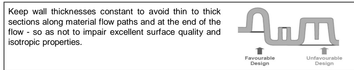
Figure 19: An example of a design recommendation adapted from the European Alliance for SMC/BMC (2007, p. 18)
