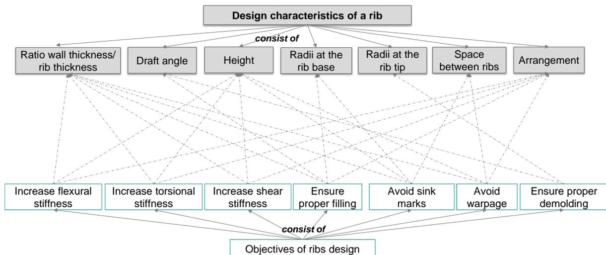
Figure 109: Model draft – an example of the rib design characteristics based on Butenko and Albers (2019, p. 284)
