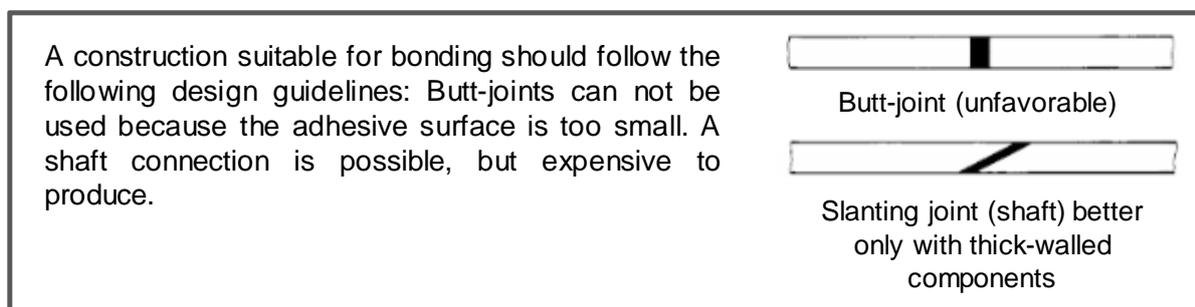
Figure 30: An example of a design guideline for bonding connections adapted from Böge and Böge (2017, p. 755)<sup>24</sup>
