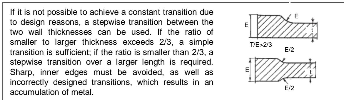
Figure 28: An example of a design guideline adapted from Verein Deutscher Giessereifachleute (2005, p. 112)<sup>22</sup>
