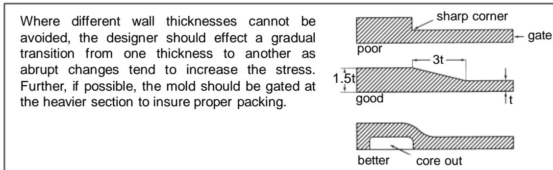
Figure 25: An example of a design guideline adapted from DuPont Engineering Polymers (2000, p. 7)
