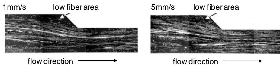
Figure 11: Influence of closing speed on fiber filling at the transition from thick-walled to thin-walled areas adapted from Schmachtenberg et al. (2005)
