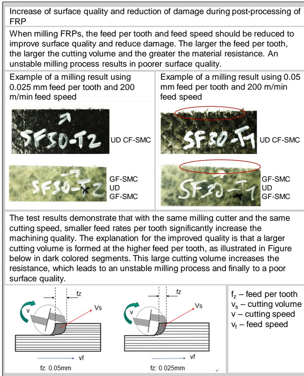
Figure 90: Created recommendation using provided guide adapted from Li 2018, p. 88<sup>144</sup>
