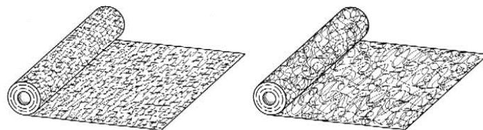
Figure 6: Example of mats with chopped and endless fibers adapted from Schürmann (2007, p. 64)
