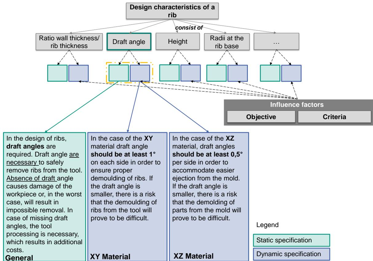
Figure 113: Static and dynamic design specifications based on Butenko and Albers (2019, p. 285)
