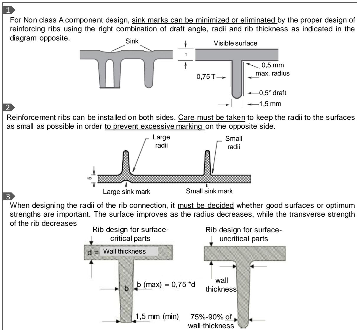
Figure 33: Comparison between three design guidelines for SMC materials on example of a rib design to avoid sink marks (1) European Alliance for SMC/BMC (2007, p. 22), (2) Wernli (1998),<sup>27</sup> (3) AVK – Industrievereinigung Verstärkte Kunststoffe e. V. (2013, p. 420)<sup>28</sup>
