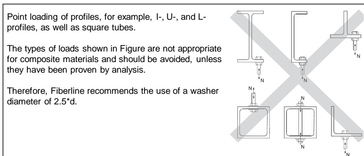
Figure 14: An example of a design guideline adapted from Fiberline Composites (2002)
