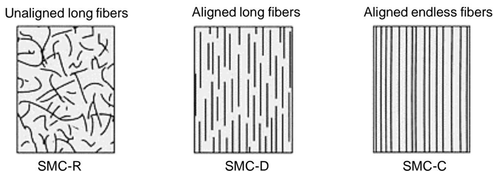
Figure 9: Designation of various SMC types adapted from Bonten (2016, p. 336)
