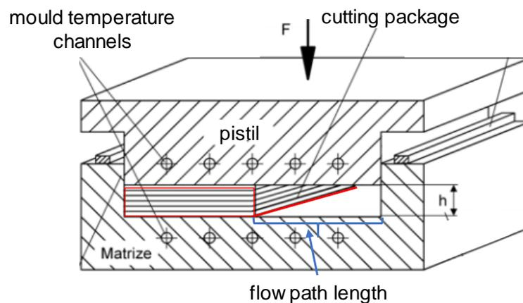
Figure 10: Initial mold coverage (in red color) adapted from Schmachtenberg et al. (2005)
