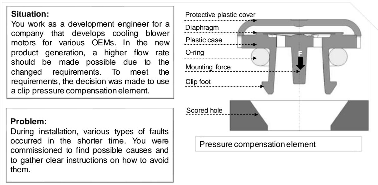
Figure 66: Example of the case study “assembly of a pressure compensation element”<sup>124</sup>
