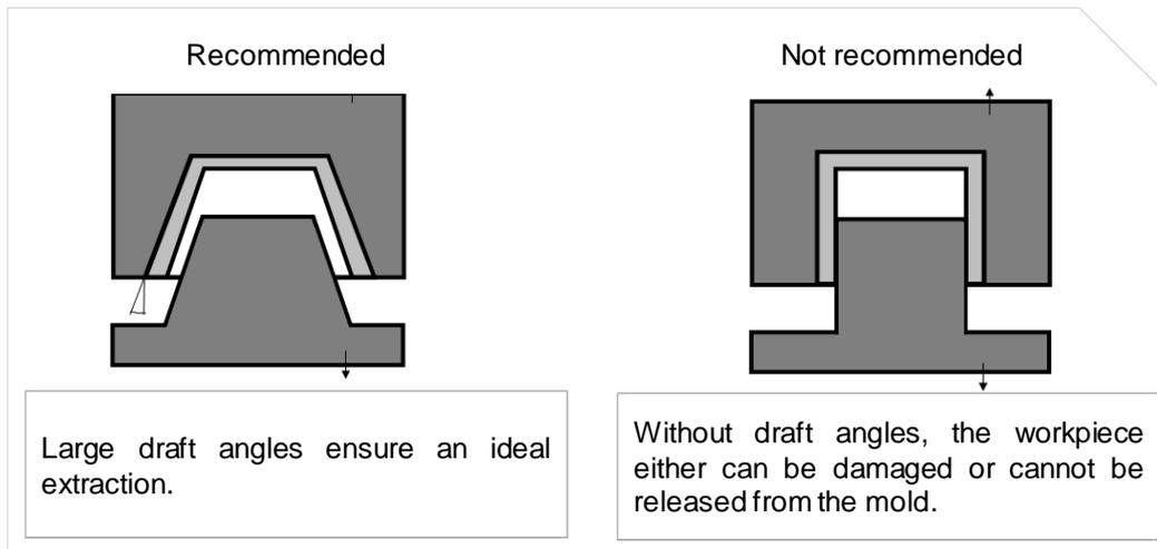
Figure 72: Recommendation in form of ideal and poor design solutions of the casting tool with brief text adapted from Butenko et al. (Butenko, Gladysz, et al., 2018)<sup>128</sup>
