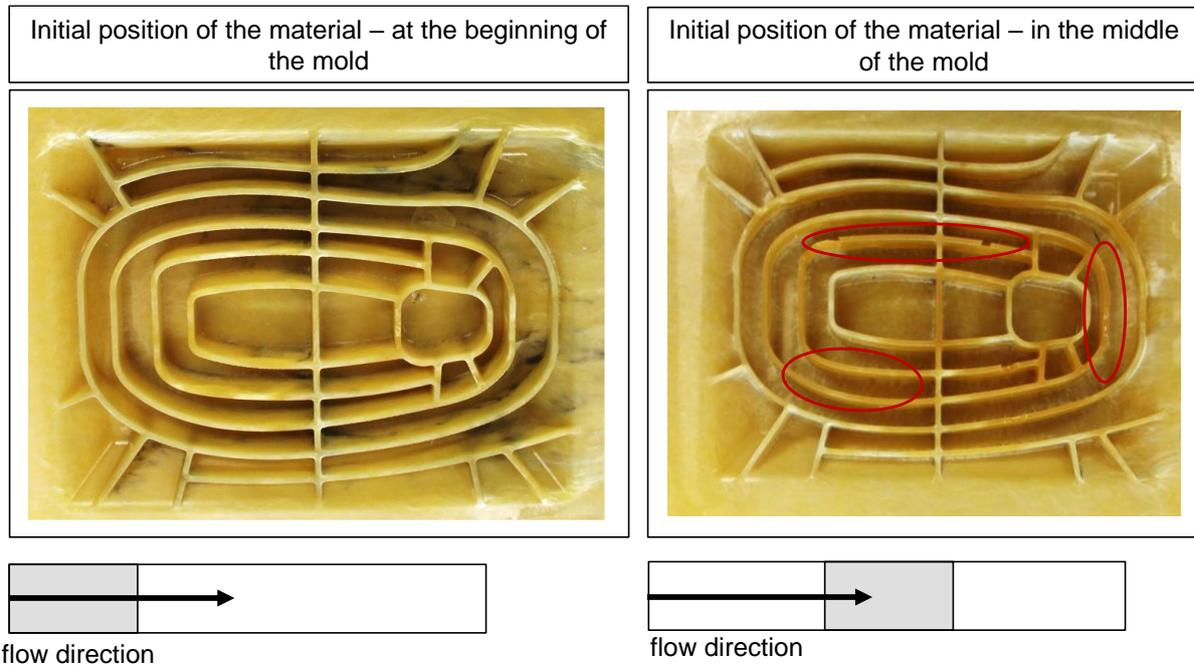
Figure 81: Influence of the initial position of the material on the rib filling<sup>139</sup>
