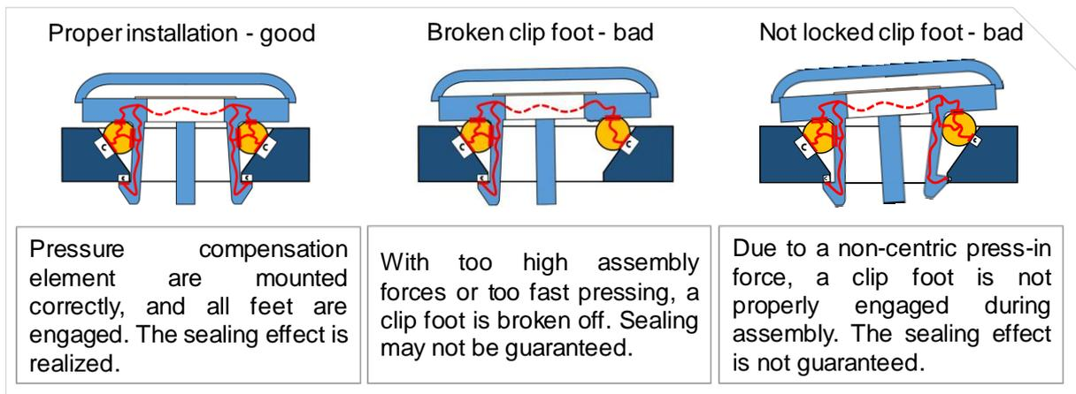
Figure 69: C&C<sup>2</sup>-based representation of ideal and poor assembly results with brief text adapted from Butenko et al. (Butenko, Gladysz, et al., 2018)<sup>126</sup>
