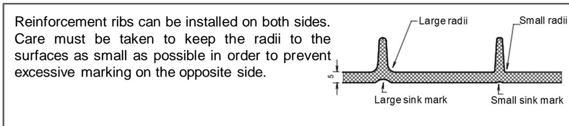
Figure 16: An example of a design guideline for SMC adapted from Wernli (1998)<sup>11</sup>
