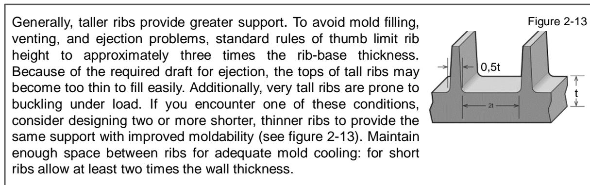
Figure 26: An example of a design guideline for unreinforced thermoplastics adapted from Lanxess Energizing Chemistry (2007)
