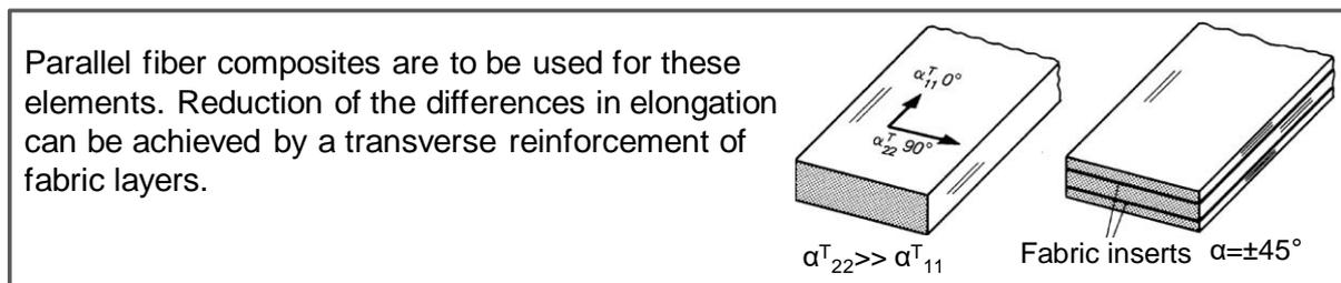
Figure 23: An example of a design guideline adapted from VDI (Verein Deutscher Ingenieure, 2014, p. 8)<sup>20</sup>
