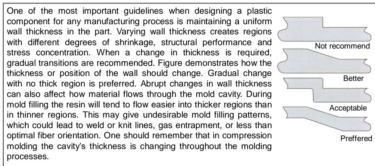
Figure 17: An example of a design guideline adapted from Davis et al. (2003, p. 113)
