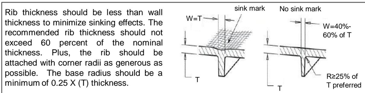
Figure 27: An example of a design guideline for unreinforced thermoplastics adapted from Stratasys Direct (2015, p. 4)
