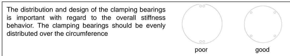
Figure 29: An example of a design guideline for sheet metals adapted from Gerd and Reitter (2013)<sup>23</sup>
