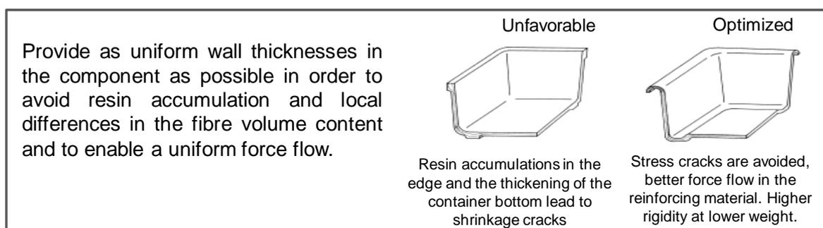
Figure 24: An example of a design guidelines adapted from Drechsler and Bockelmann (2016, p. 890)<sup>21</sup>
