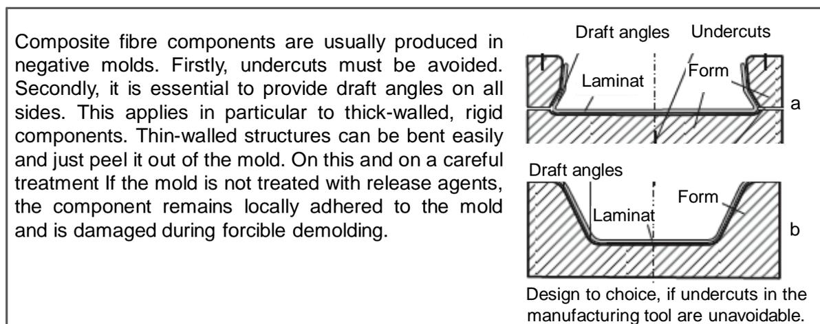
Figure 18: An example of a design guideline adapted from Schürmann (2007, p. 624)<sup>13</sup>
