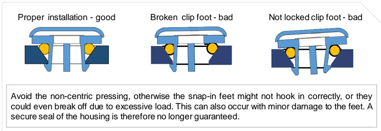
Figure 68: Recommendation in form of ideal and poor assembly results with the brief explanatory text adapted from Butenko et al. (Butenko, Gladysz, et al., 2018)<sup>125</sup>
