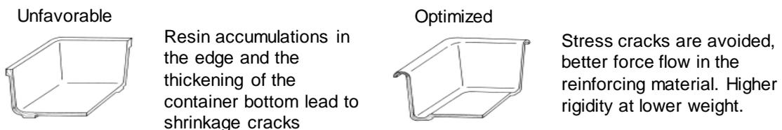
Figure 31: Comparison among four design guidelines for FRPs for the example of topic wall thickness adapted from (1) Davis et al. (2003, p. 113), (2) the European Alliance for SMC/BMC, (2007, p. 18), (3) AVK – Industrievereinigung Verstärkte Kunststoffe e. V. (2013, p. 419),<sup>25</sup> and (4) Drechsler & Bockelmann (2016, p. 890)<sup>26</sup>
