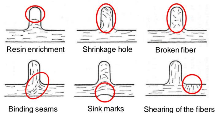
Figure 13: Fiber content and fiber orientation inhomogeneities in the rib area adapted from Specker et al. (1990, p. 86)
