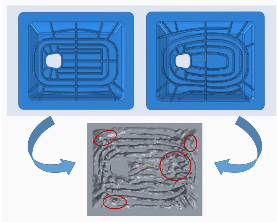
Figure 77: Design solutions for rib based on topology optimization (left – the first solution and right – the second solution)<sup>134</sup>
