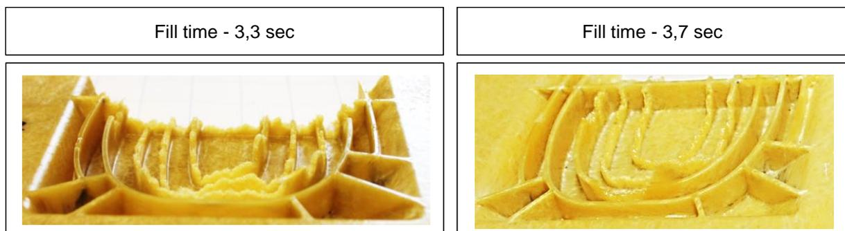
Figure 80: Fill time of 3.3 and 3.7 seconds – shaping of the rib<sup>138</sup>
