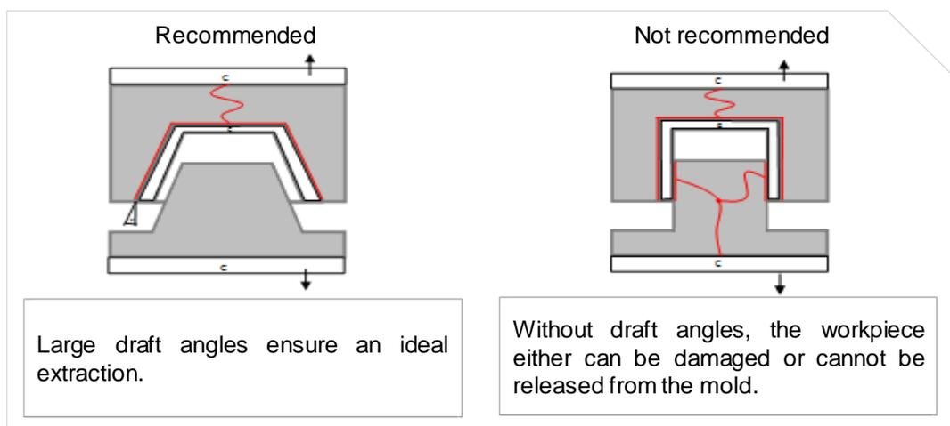
Figure 73: C&C<sup>2</sup>-based representation of ideal and poor design solutions with brief text adapted from Butenko et al. (Butenko, Gladysz, et al., 2018)<sup>129</sup>
