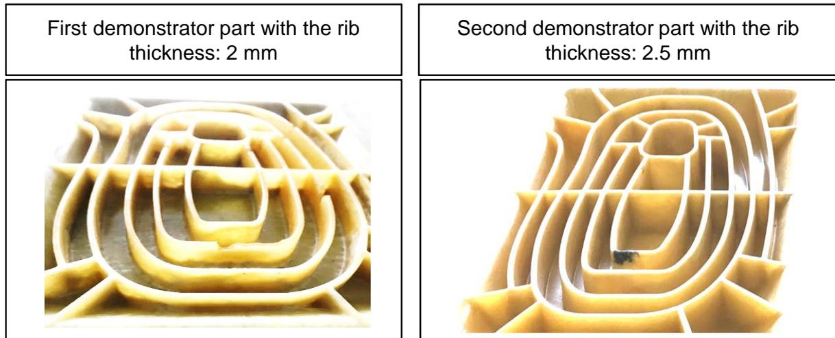
Figure 82: Comparison of first and second demonstrators – improved rib filling adapted from Butenko and Albers (2019, p. 280)<sup>140</sup>
