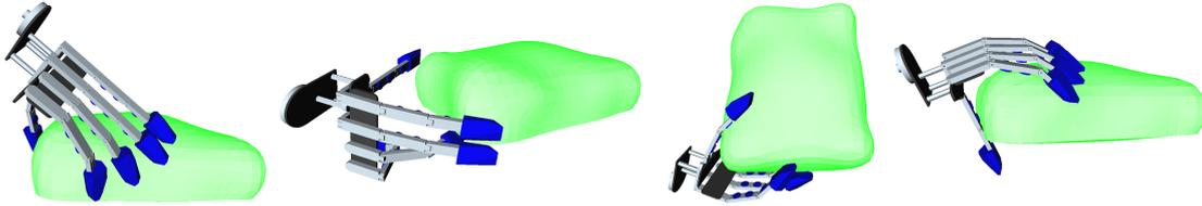
Figure 3.23: Grasp candidates generated by the surface based grasp planner.
