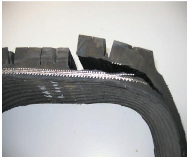
**Figure 1.4:** Cross-section view of a failure truck tire after a durability test [31].
