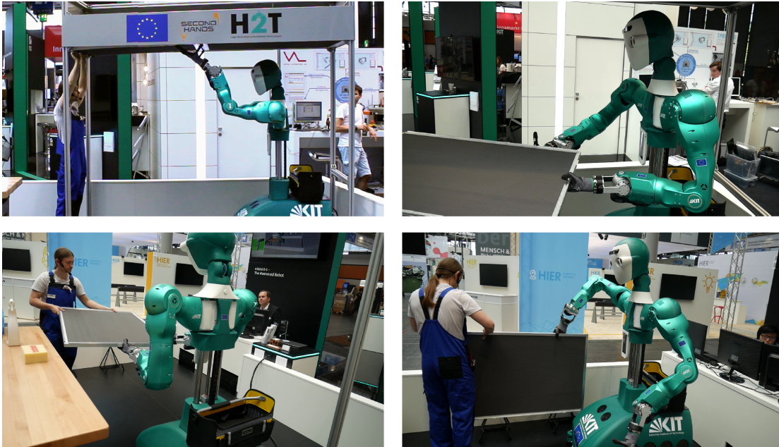
Figure 5.4.: The technician and ARMAR-6 remove the cover panel in a cooperative bi-manual mobile manipulation task. Source: (Asfour et al., 2018) © 2018 IEEE.
