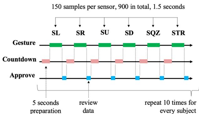
**Figure 6: The graph shows the structure of the data acquisition session. Participants perform each gesture after a five-second preparation time. We review the recorded samples immediately and then manually start the next countdown.**
