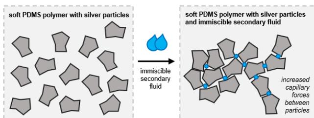
**Figure 1:** The schematic drawing shows how the secondary immiscible fluid improves the capillary forces between silver particles. The illustration was adapted from the work by Sun et al. [25].
