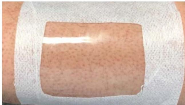
**Figure 10: The patch firmly pulls the PDMS substrate material onto the user’s skin on the forearm to enable a soft interactive surface that naturally blends in.**
