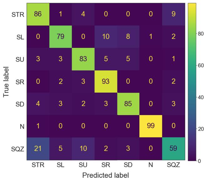
**Figure 9: Leave one subject out confusion matrix showing that squeezing and stretching is most challenging to classify in our limited resolution sensor setup.**
