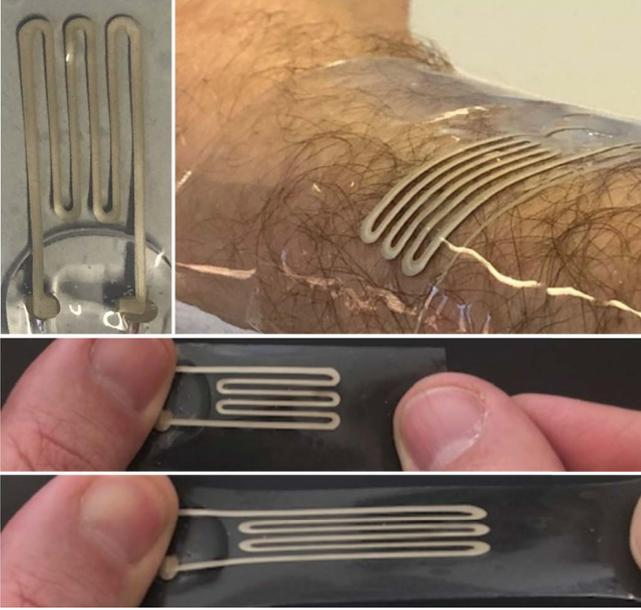
**Figure 3:** The upper left image shows a resistor made from capillary Ag-PDMS. The top right image displays how the material applies to the arm, leaving almost no gap between the PDMS base layer and the skin. Even long hair tightly fits between the substrate and the arm. The two images in the bottom show the stretchability of the material, which keeps its electric properties for an intense stretch of  $\gg 100\text{--}200\%$ .
