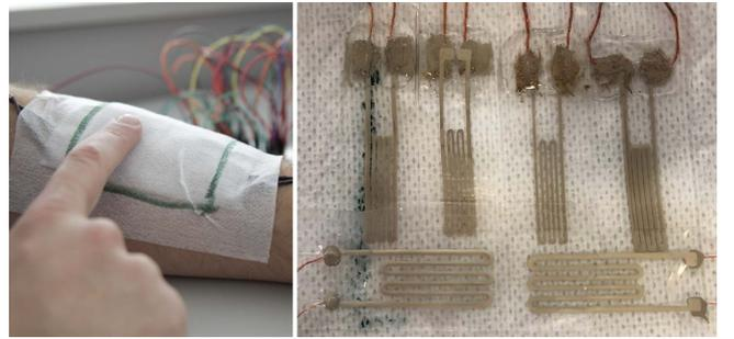
**Figure 4:** Our prototype device consists of six stretchable sensors that we affixed with medical adhesive tape.
