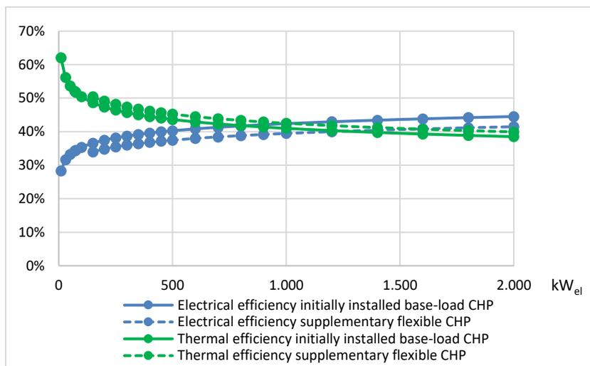
Figure A. 15: Thermal and electric CHPs efficiency for base-load CHPs and supplementary flexible CHPs as a function of the installed electric power [150]
