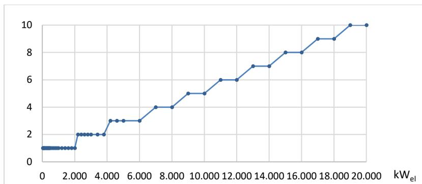
Figure A. 16: Number of CHP gas engines as a function of the installed electric power
