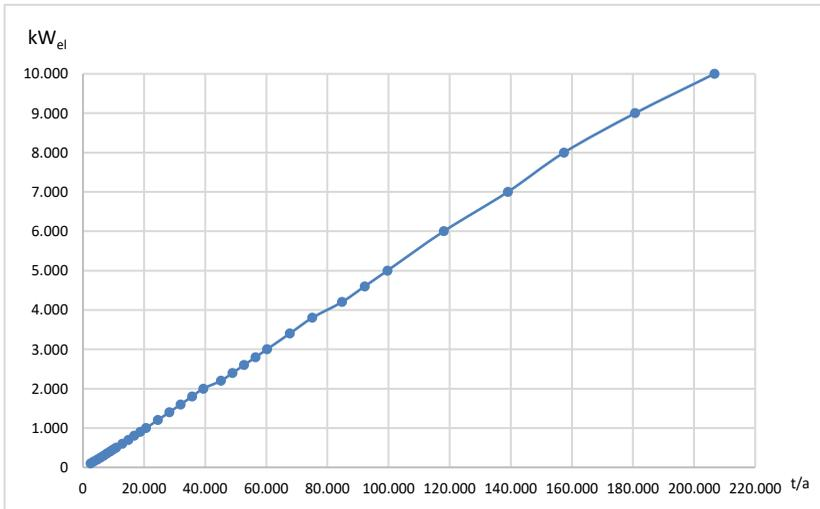
Figure 4.4: Correlation between the CHP-electric power and the biomass input mass flow
