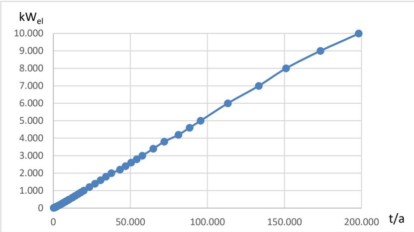
Figure A. 5: Electric power as a function of the biomass input mass flow (E plant)
