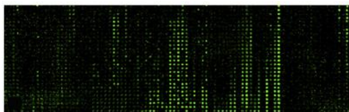
Figure 3. Fluorescence image of a 2280-membered library with captured fluorescent HeLa cells. Cell numbers calculated at different temperatures correlate with polymer composition and temperature. Reproduced from 65
