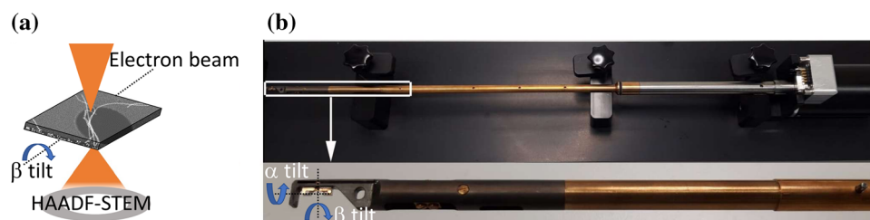
Figure 2 a Simplified scheme of HAADF-STEM tomography. b Photograph of STEM sample holder of the Helios G4 FX. The front region of the rod (marked by a white rectangle) is magnified in the photograph below with \alpha -tilt and \beta -tilt directions indicated.
