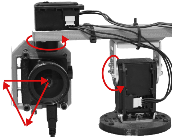
Figure 6.1.: Microsaccadic motion of the DVS performed by the robotic head. Source: [6].
