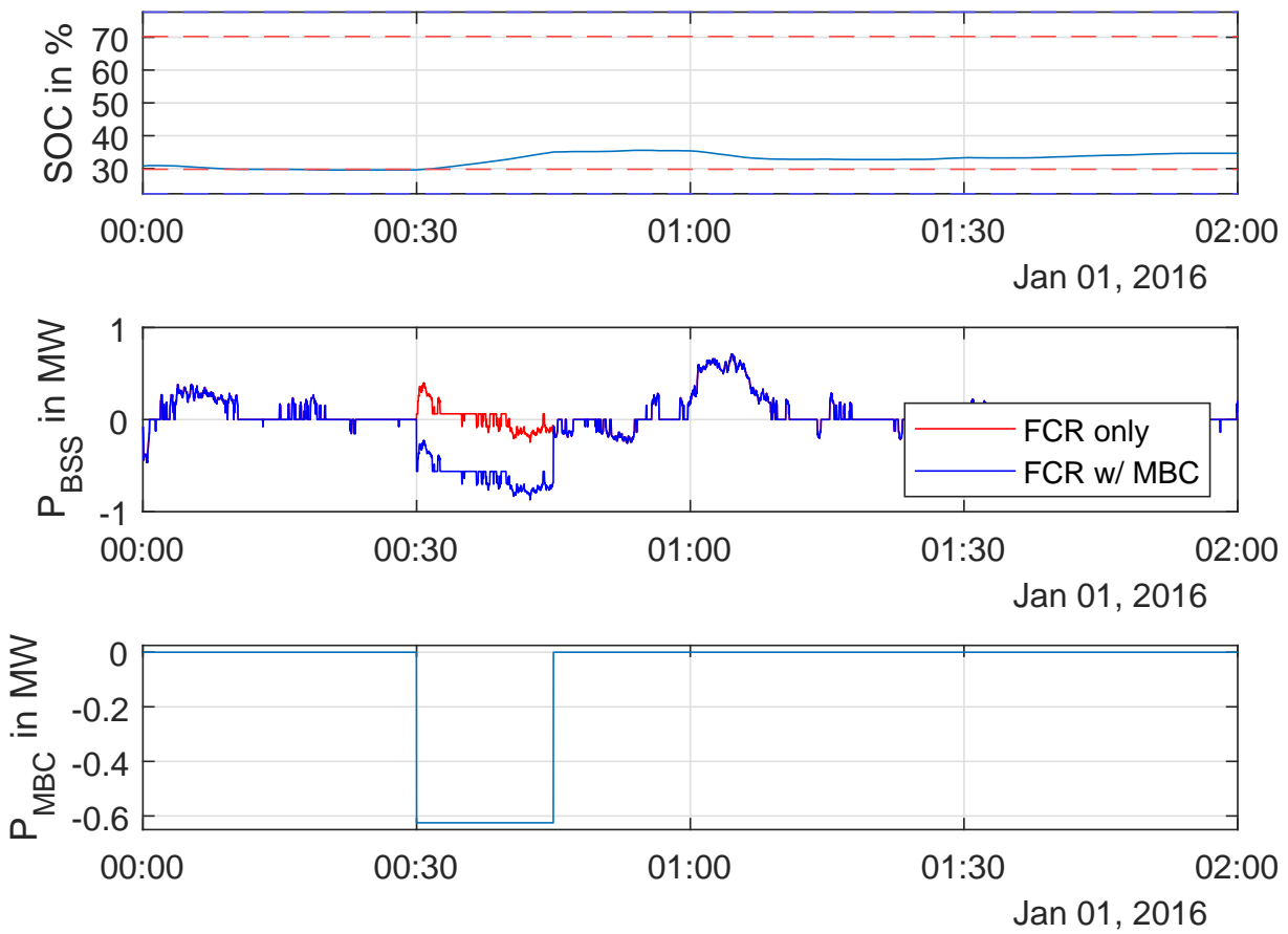
Figure 5.9: Example of charge management for charge of BSS while simultaneously providing FCR The figure shows on the y-axis SOC development in the top graph, requested FCR power P_t^{FCR\_request} (FCR only) and final power P_t (FCR w/ MBC) in the center graph, and MBC in the bottom graph for two hours of FCR provision on the x-axis
