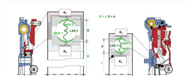
Figure 2 – EV using the DMS rolling bearing as an example [16] (figure adapted). Blue is the primary mass of the DMF, red the secondary mass, yellow are the coil springs between the two masses.
