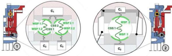
Figure 3 - PV: Change of the bearing principle in the second product generation of dual mass flywheels (DMF) as described in [16] (figure adapted). Blue is the primary mass of the DMF, red the secondary mass, yellow are the coil springs between the two masses.
