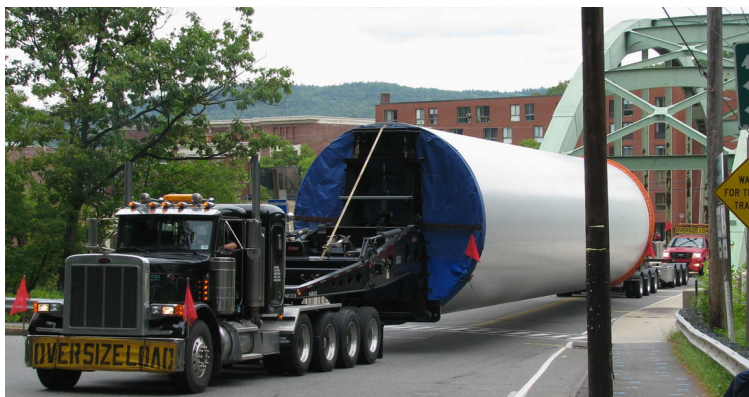
Figure 2.10: Tower section transport under the 1935 Ramford bridge [116]
