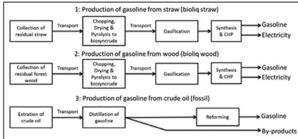
**Fig. 1.** Considered fuel production routes: bioliq straw (1), bioliq wood (2), fossil (3).
