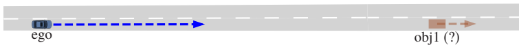
Figure 5.10: Ghost object scenario: There is an uncertain vehicle detection ahead in the ego lane.
