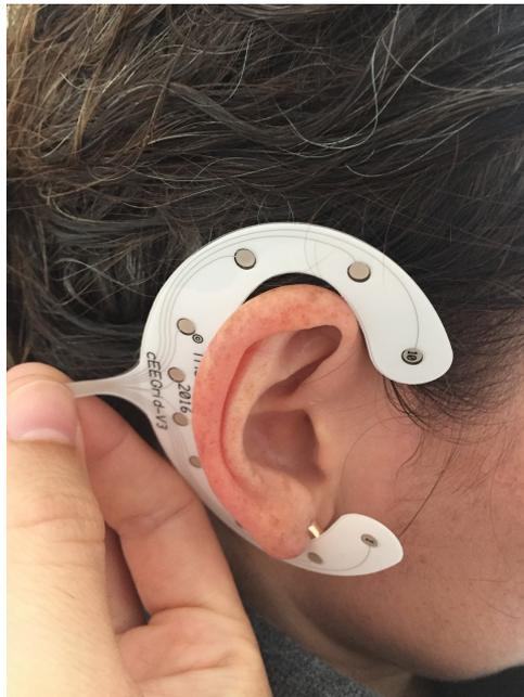
FIGURE 8.1: cEEGrid - A Flexible EEG Array With Ag/AgCl Electrodes That Can Be Placed Around the Ear Using Adhesives.
