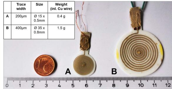
**Figure 3: Different diameters and trace width/distance**
