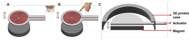
**Figure 6: (A). Observe; (B). Hover; (C). Section view of 3D printed case.**
