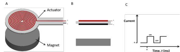
**Figure 1: (A). 3D view of the FLECTILE with printed coils designed in clockwise and counterclockwise on two sides of the substrate; (B). Front view of the FLECTILE ; (C). Driving method: 5V DC power switching on and off.**
