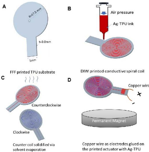
**Figure 2: (A).** print a TPU substrate with a 1mm all-through hole in the center; **(B).** print capillary Ag-TPU ink traces on both sides of the substrate; **(C).** cure the trace; **(D).** connect copper wires and trace using the same Ag-TPU ink.
