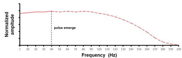
**Figure 4: Exp. 1, Actuator response frequency: 1-200Hz**
