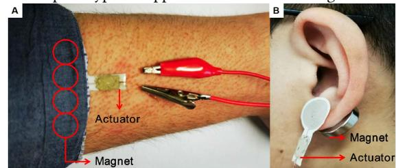
**Figure 7: Application:(A). Vibration sleeves; (B). Earring-shaped haptic feedback system.**
