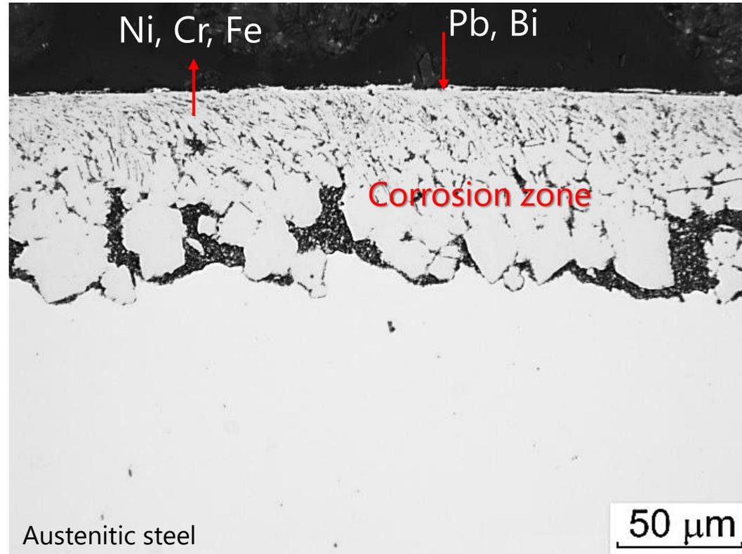
Pure Pb-Bi de-alloys intensively steels at high temperatures
