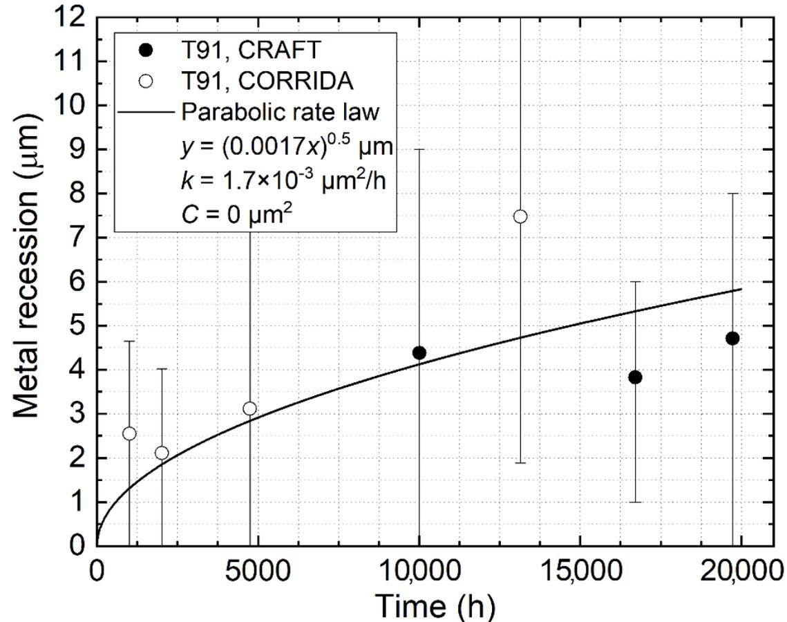
Corrosion rate  $\sim 4 \mu\text{m}/\text{year}$
