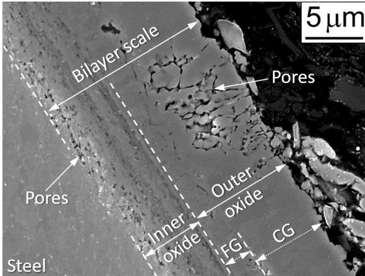
Bilayer magnetite scale:  $\text{Fe}_3\text{O}_4/\text{Fe}(\text{Fe},\text{Cr})_2\text{O}_4$
