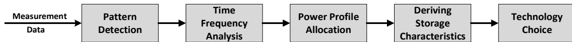
Figure 9.1 Overview of the process from raw measurement time series to storage technology choice. This process is repeated with different data resolution.
