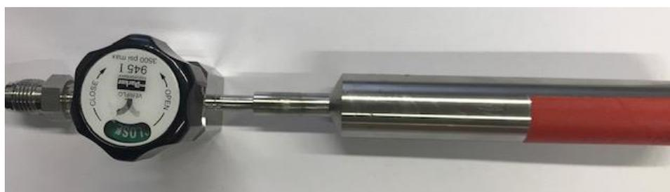
Figure 8: The gas sampling cylinder used for sampling of the gas phase.
