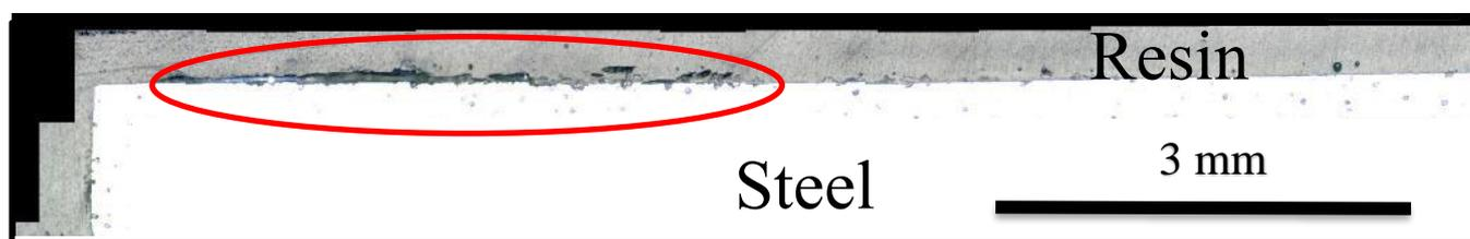
Figure 17: The optical image of the crosscut with the red circle highlighting the interface of interest in SGI sample corroded in 5 M NaCl for 31 weeks at 90 °C.
