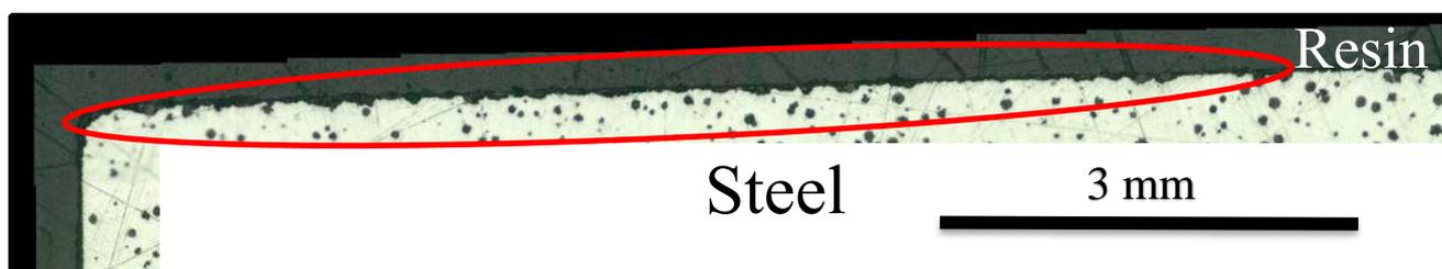
Figure 27: The optical images of the crosscut with the red circle highlighting the interface of interest for SGI sample corroded in 3.4 M  $\text{MgCl}_2$  for 31 weeks at 90 °C.
