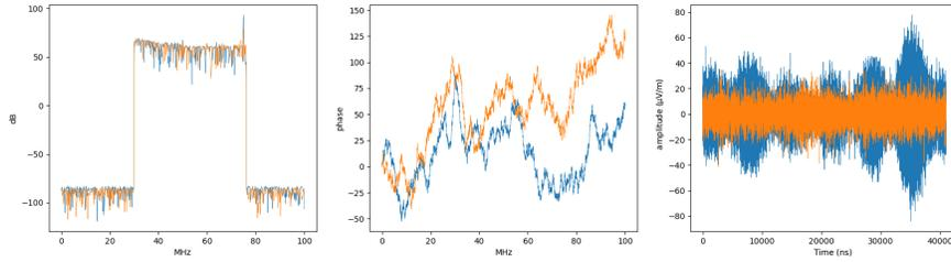
**Fig. 3.** Example of generated noise. From left to right: spectra, phases, resulting traces.
