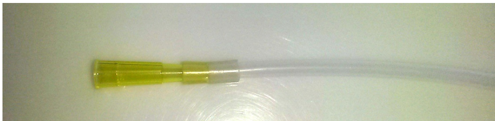
Figure 6.18: Assembled pipette tip filler to transfer freely swollen gels.
