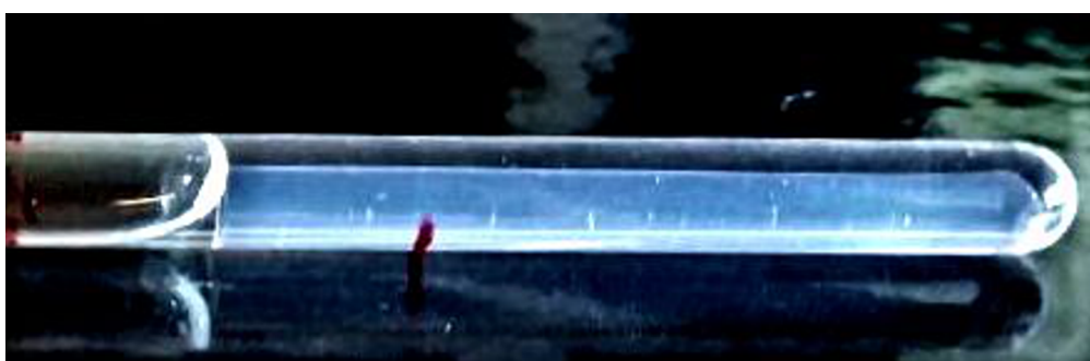
Figure 5.6: PMMA gel stick in chloroform with inner cracks due to fast swelling.
