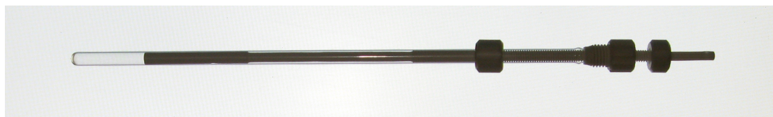
Figure 5.4: Compressing apparatus, consisting from a special NMR tube with a burl on top and screw nuts to fix the teflon ® plunger at a certain height.
