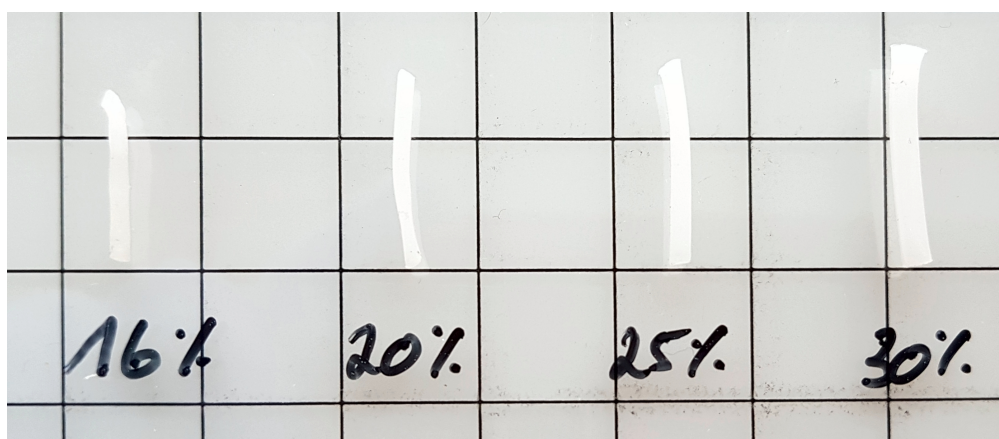
Figure 6.14: Cross-linked PEO-DA sticks with different polymerization mass contents (%(w/w)) after vertical drying.
