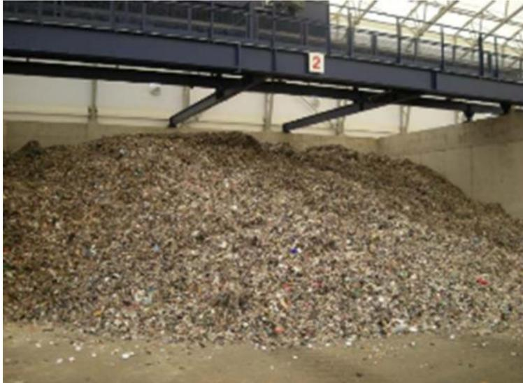
Figure 5: Certificated Solid Recovered Fuel (SRF) produced from biomass and household waste in the frame of the EU funded RECOMBIO project [Gehrmann et al., 2018]
