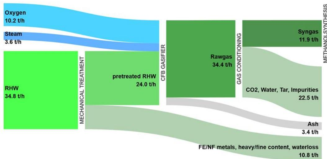
Figure 9: material flows in the process chain “fluidized bed gasification of residual household waste”. Heat load of the gasification step is 100 MW.
