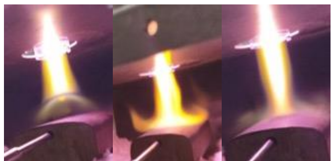
Figure 6: Effect of gas flow on plasma afterglow delivery at 2kW
