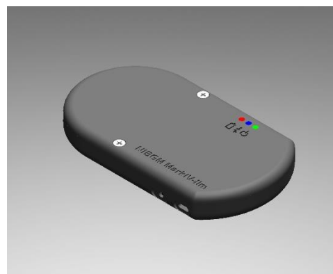
Figure 4: The microwave non-invasive blood glucose sensor
