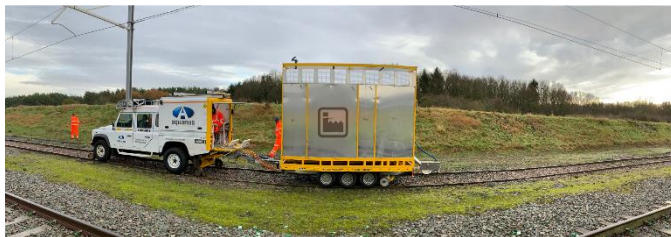
Figure 2: Road-Rail Demonstrator Prototype on UK Rail Network
